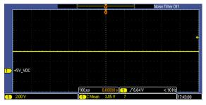
Figure 111. 5.0V\_VDC Power Rail on DSM Board
