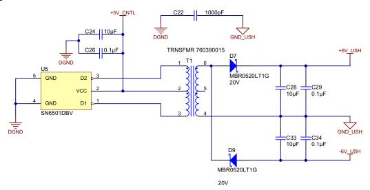
Figure 36. SN6501-Based Power Isolation
