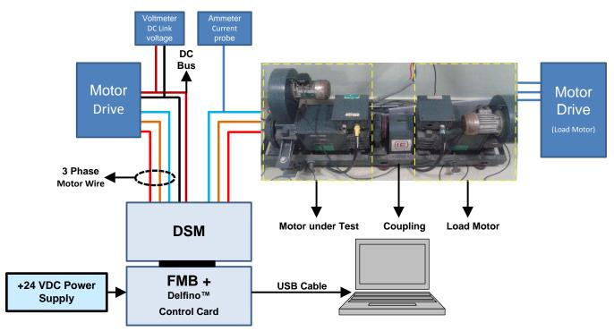
Figure 93. Test with Motor Drive and Load Setup
