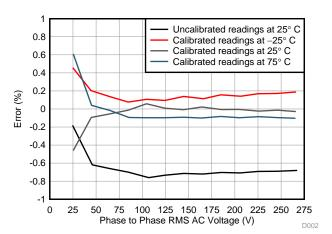
Figure 83. Phase-to-Phase Voltage versus Error with In-Amp
