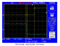
Figure 98. Short Circuit Signal Applied to AMC1304 (Blue) and Signal From MCU (Yellow) on GPIO1 Pin 10 on J2 Header on FMB Board
