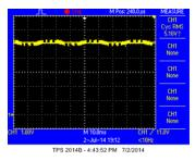
Figure 126. 5.0V\_USH Power Rail on DSM Board, Measured Across Capacitor C38, with Motor Turned On
