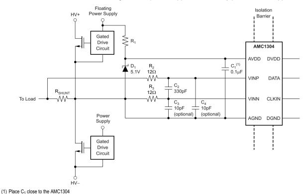
Figure 39. AMC1304 Biasing from Gate-Drive Power Supply
