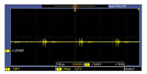
Figure 106. 1.25-V Reference Voltage from REF3012, on FMB Board
