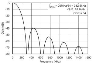
Figure 10. Magnitude versus Frequency Response of the Sinc<sup>3</sup> Filter
