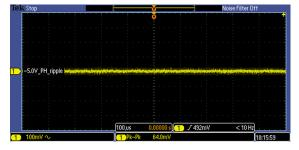
Figure 117. Ripple on –5.0V\_PH Power Rail on DSM Board, Measured Across Capacitor C84, with Motor Turned On
