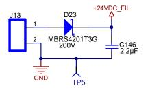
**Figure 42. Input Polarity Protection**
