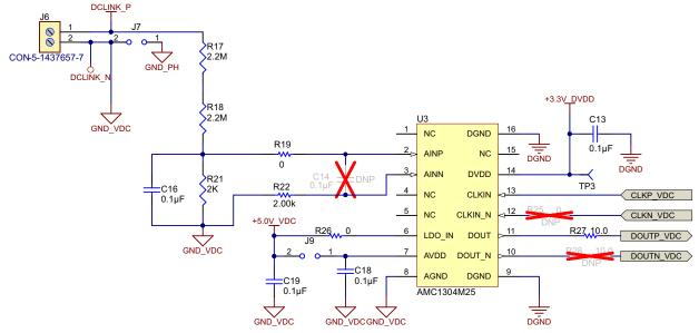
The jumper (J7) needs to be disconnected to perform this measurement.
