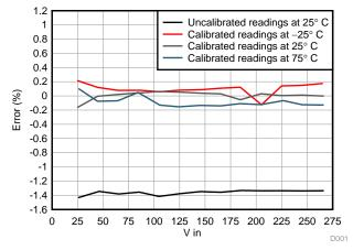
Figure 82. Phase-to-Phase Voltage versus Error
