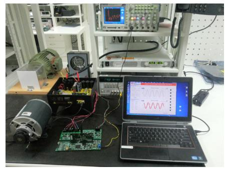
Figure 99. Isolated Current Shunt and Voltage Measurement Eval Kit with HV Invertor Kit and AC Motor
