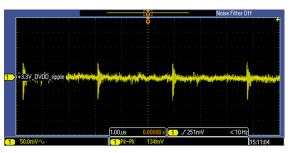
Figure 105. Ripple on 3.3V\_DVDD Power Rail, on FMB Board
