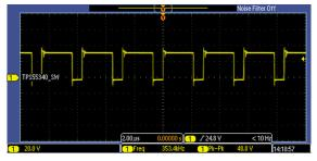
Figure 100. Switch Node Wave Form for TPS5534 24 V to 6 V, DC-DC Converter
