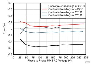
Figure 84. Phase-to-Phase Voltage versus Error with In-Amp and Sallen Key
