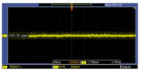
Figure 115. Ripple on 5.0V\_PH Power Rail on DSM Board, Measured Across Capacitor C103, with Motor Turned On
