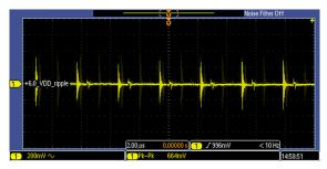
Figure 102. Ripple on 6.0\_VDD Power Rail, FMB Board
