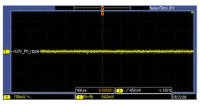
Figure 121. Ripple on –6V\_PH Power Rail on DSM Board, Measured Across Capacitor C83, with Motor Turned On
