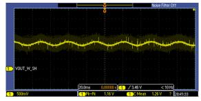
Figure 132. DAC Output, VOUT\_W\_SH, with Shunt Value of 5 m $\Omega$
