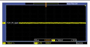
Figure 116. –5.0V\_PH Power Rail on DSM Board, Measured Across Capacitor C84, with Motor Turned On
