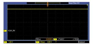
Figure 114. 5.0V\_PH Power Rail on DSM Board, Measured Across Capacitor C103, with Motor Turned On
