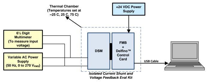
Figure 81. Test Setup for AC Voltage Measurement Accuracy
