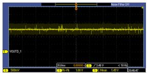
Figure 134. DAC Output, VOUTD\_1; Represents the DC Link Voltage; DC Link Voltage was 150 V
