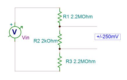
Figure 28. Phase-to-Phase Resistor Divider
