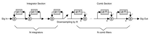
Figure 7. CIC Filter Structure
