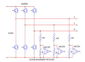
Figure 27. AMC1304 for Phase-to-DC\_MINUS Voltage Measurement
