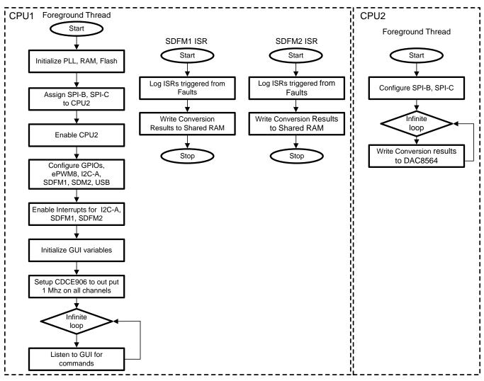
Figure 59 shows the firmware flow graph and arrangement of tasks between CPU1 and CPU2.
