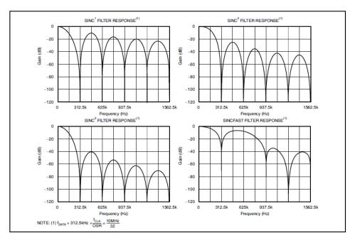
Figure 58. Frequency Response of Various Sinc Filters
