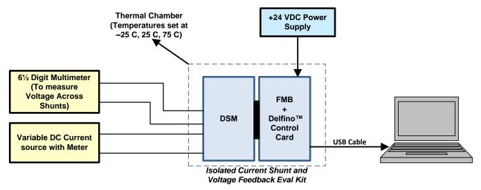
Figure 89. Test Setup for DC Measurement Accuracy
