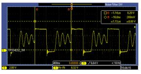
Figure 103. Switch Node Waveform for TPS54232, 6-V to 3.3-V DC-DC Converter, on FMB Board
