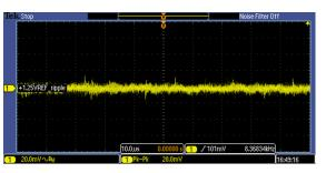
Figure 107. Ripple on 1.25-V Reference Voltage from REF3012, on FMB Board
