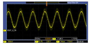
Figure 133. DAC Output, VOUT\_U\_SH, with Shunt Value of 50  $m\Omega$
