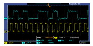
Figure 131. Data out of AMC1304 (Blue Wave Form) and Input Clock (Yellow Wave Form)
