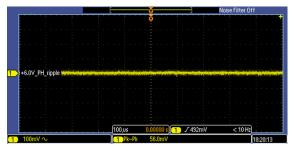
Figure 119. Ripple on  $6V_PH$  Power Rail on DSM Board, Measured Across Capacitor C107, with Motor Turned On
