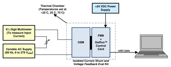
Figure 91. Test Setup for AC Current Measurement Accuracy
