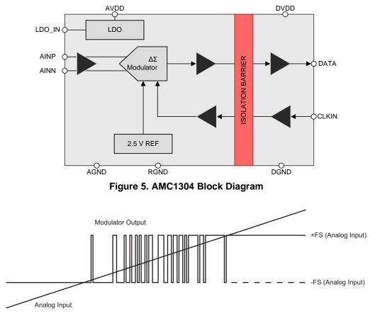
Figure 6. AMC130x Input Voltage versus Output
