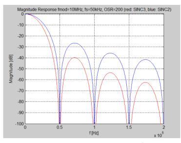
Figure 11. Magnitude versus Frequency Response of Sinc<sup>2</sup> Compared to Sinc<sup>3</sup> Filter
