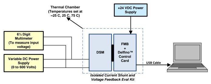
Figure 86. Test Setup for DC Link Voltage Measurement Accuracy
