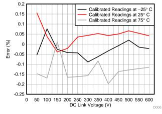
Figure 88. DC Link Voltage versus Error
