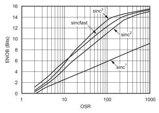
Figure 12. Measured Effective Number of Bits versus Oversampling Ratio
