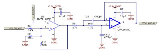
Figure 51. Amplifier and Sallen-Key Filter
