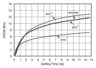
Figure 13. Measured Effective Number of Bits versus Settling Time
