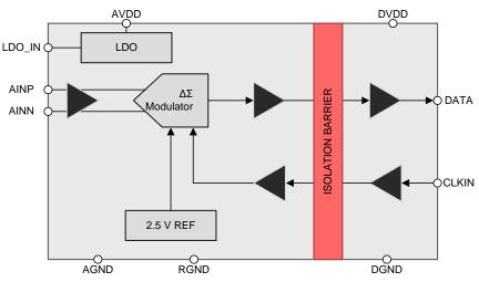
Figure 35. Block Diagram for AMC1304
