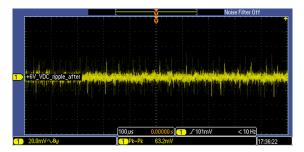
Figure 110. Ripple on 6.0V\_VDC Power Rail on DSM Board, Measured Across Capacitor C73, with Motor Turned On
