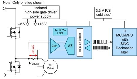
Figure 2. Delta-Sigma Modulator in Three-Phase Inverter
