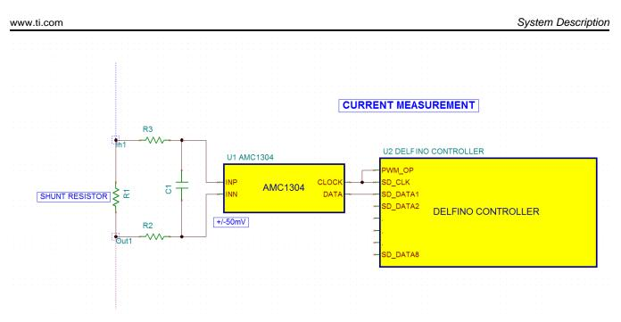
Figure 3. Current Measurement Using AMC130x and Delfino Controller
