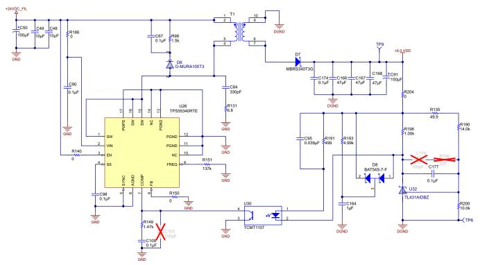
Figure 43. 24-V DC to 6-V DC Flyback Convertor
