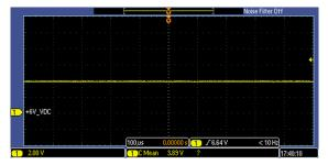
Figure 108. 6V\_VDC Power Rail on DSM Board, Measured Across Capacitor C73
