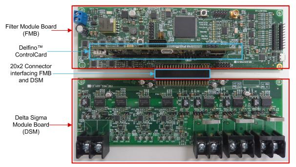
Figure 14. Picture of Isolated Current and Voltage Measurement Kit
