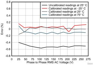
Figure 85. Phase-to-DC\_MINUS versus Error with Sallen Key
