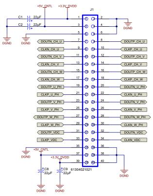
Figure 41. Board-to-Board Connector
