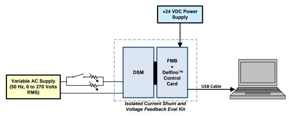
Figure 96. Test Setup for Short Circuit Testing
