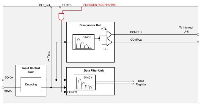
Figure 57. Block Diagram of One Filter Module
