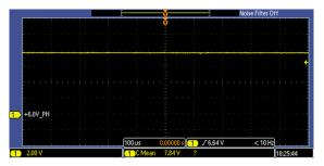
Figure 118. 6.0V\_PH Power Rail on DSM Board, Measured Across Capacitor C107, with Motor Turned On
