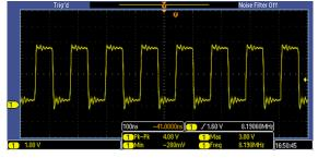
Figure 130. Input Clock to AMC1304
