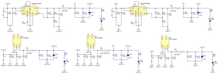
Figure 138. Power Supply 2 Schematic
