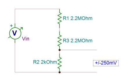
Figure 32. Phase-to-DC\_MINUS Resistor Divider
