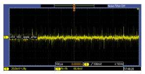
Figure 113. Ripple on 5.0V\_PH Power Rail on DSM Board, Measured Across Capacitor C96, with Motor Turned On
