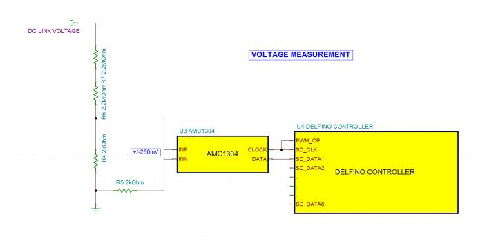
Figure 4. Voltage Measurement Using AMC130x and Delfino Controller
