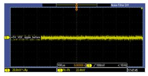
Figure 112. Ripple on 5.0V\_PH Power Rail on DSM Board, Measured Across Capacitor C96, with Motor Turned Off
