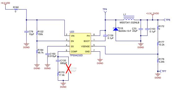
Figure 46. 6- to 3.3-V Step Down Convertor
