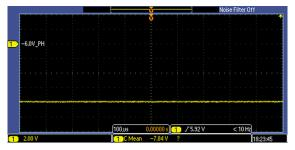
Figure 120. –6.0V\_PH Power Rail on DSM Board, Measured Across Capacitor C83, with Motor Turned On
