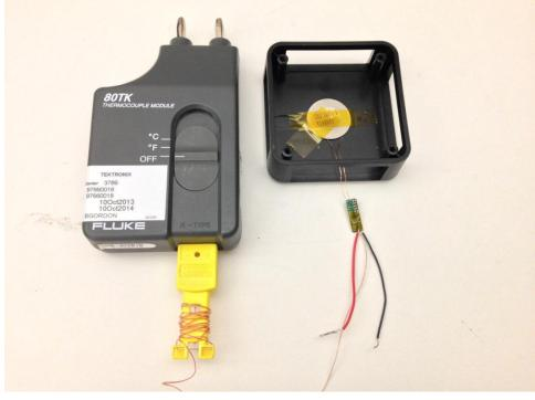
Figure 6. FLUKE 80TK Thermal Couple
