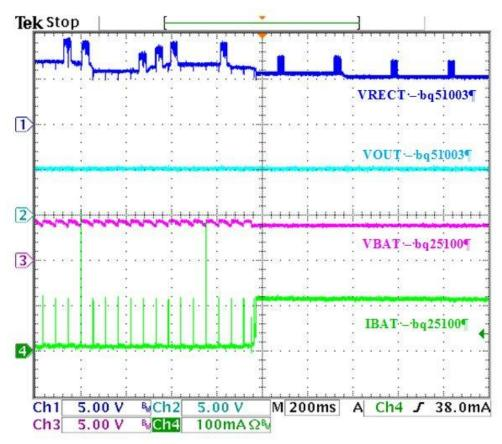
Figure 11. IBAT Load Transition from 0 mA to 100 mA
