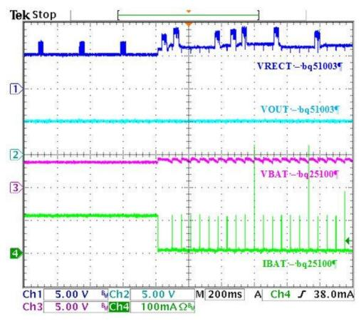
Figure12. IBAT Load Transition from 100 mA to 0 mA
