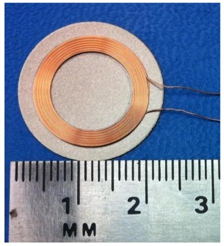
Figure 3. Receiver Coil
