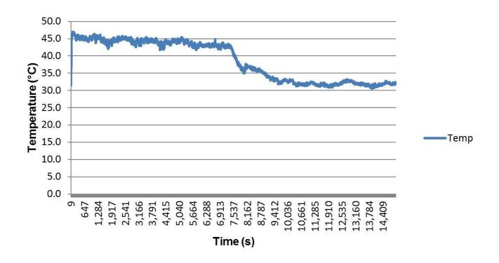
Figure 10. 4.2 V 60 mA Charge Cycle with 1 mA Charge Termination (2)
