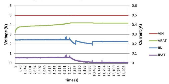
4.2 V 60 mA Charge Cycle with 1 mA Charge Termination
