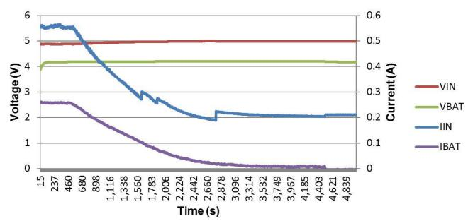
4.2 V 250 mA Charge Cycle with 10 mA Charge Termination
