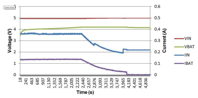
Figure 8. 4.2 V 135 mA Charge Cycle with 20 mA Charge Termination
