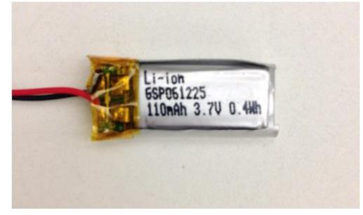
Figure 5. 110 mAh Li-Ion Battery Pack
