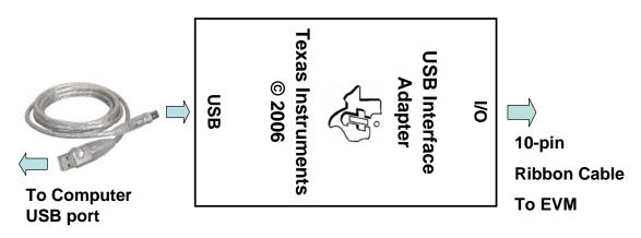
Figure 1. Connections of the HPA172 kit.
