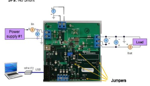
Figure 2. Original test setup for TIDA-00036 (bq2419x EVM).
