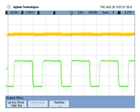
Figure 26 2.8V Output Ripple at 2A Load
