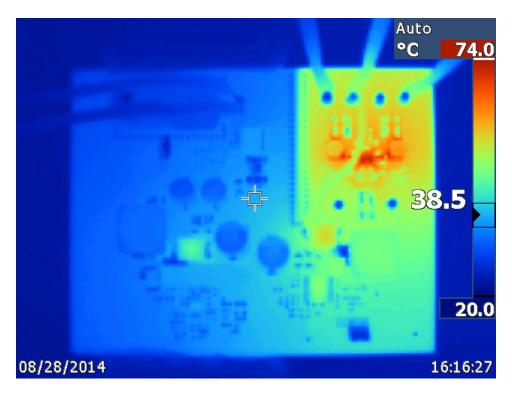
Figure 4 Board Thermal Image at 12V input
