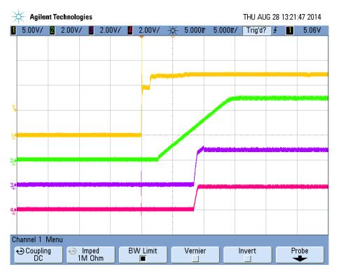
Figure 20 Start Up into No Load at 12Vin
