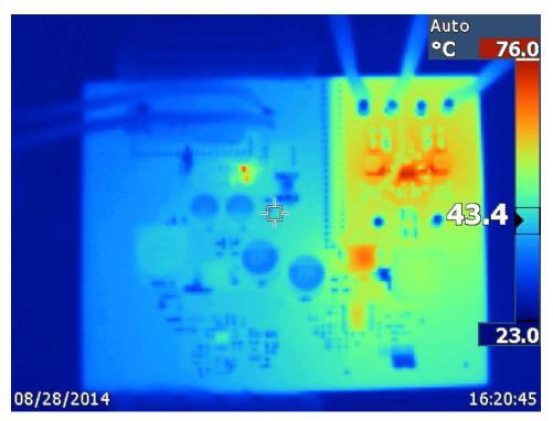
Figure 5 Board Thermal Image at 38V input
