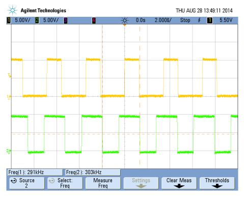
Figure 9 Switching Waveforms for the Pre-boost and the 5V Buck at 4.5Vin and 2A Load
