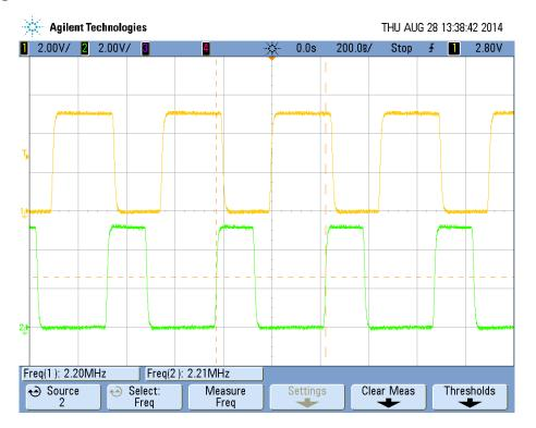
Figure 14 Switch Node Waveforms for the 2.8V and 1.8V Buck at No Load
