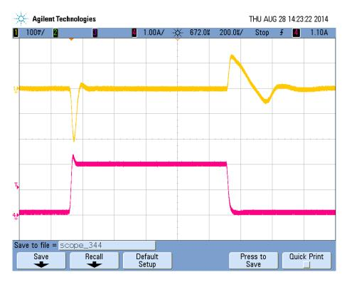
Figure 21 5V Output Buck Regulator Load Transient
