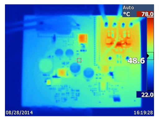
Figure 3 Board Thermal Image at 4.5V input
