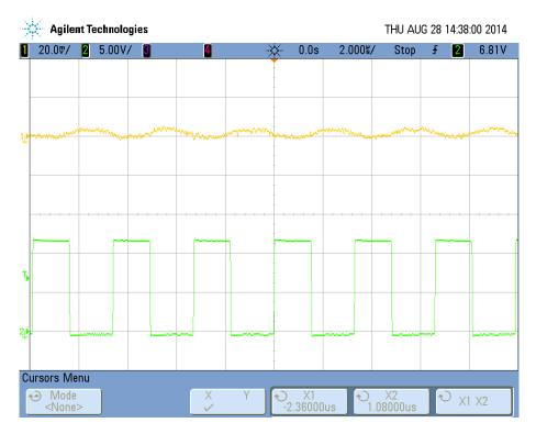
Figure 24 5V Output Ripple at 2A Load, 12Vin
