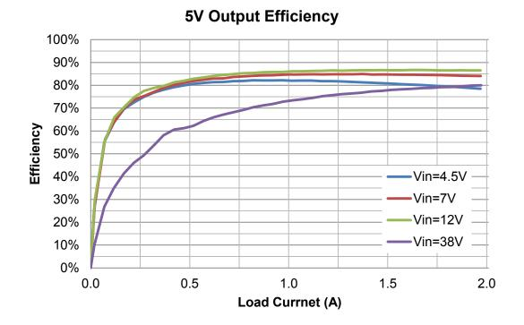
Figure 6 5V Output Efficiency
