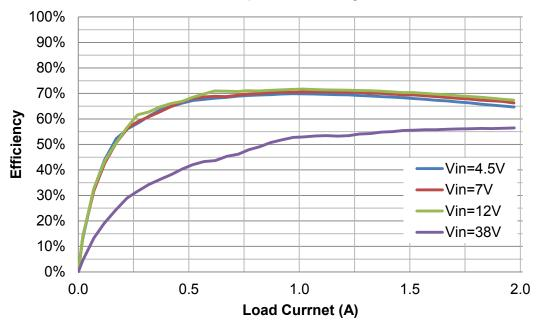
Figure 8 1.8V Output Efficiency
