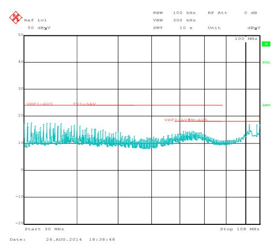
Figure 18 Average detect, 30MHz – 108MHz
