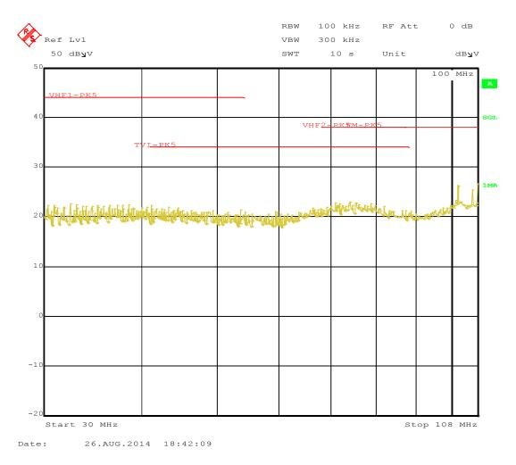
Figure 17 Peak detect, 30MHz – 108MHz
