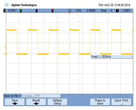
Figure 11 Switching Waveform for the 5V Buck at 12Vin and 2A Load
