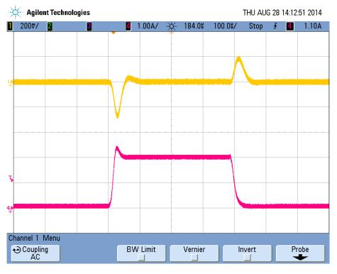
Figure 22 2.8V Output Buck Regulator Load Transient
