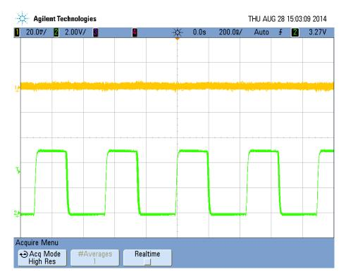
Figure 27 1.8V Output Ripple at 2A Load
