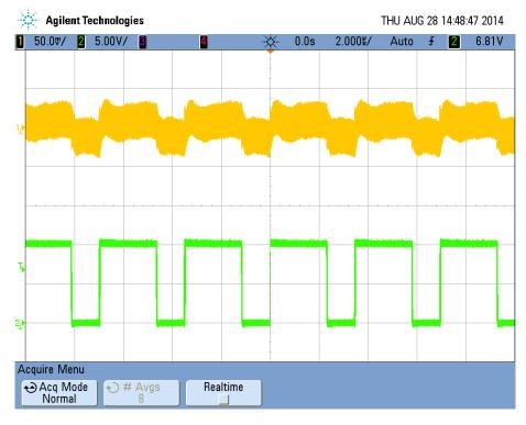
Figure 25 Pre-boost Output Ripple at 4.5Vin, 2A Load at 5Vo
