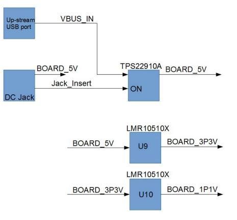
Figure 5. Power Sub-System Block Diagram
