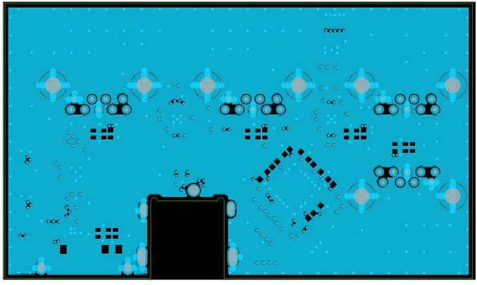
Figure 7. Layer 2 – Ground Plane
