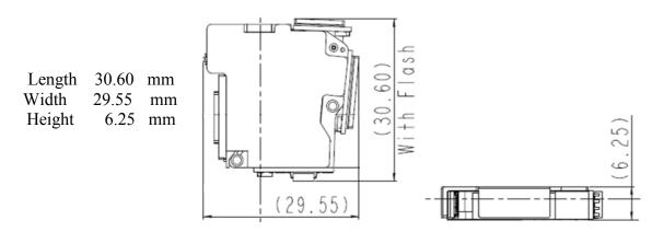
Total volume of the optical engine is: 4-6 cc Weight of the optical engine: 15 gram.
