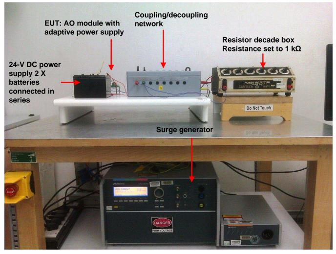
Figure 27. Surge Test Setup
