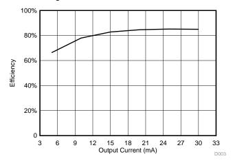
Figure 22. Boost Converter Output Current versus Efficiency
