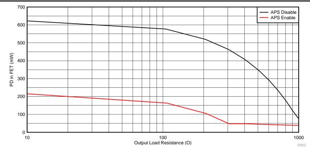
Figure 24. Output Current versus Power Dissipation in FET (Load Resistor Sweep From 10 to 1000 Ω)
