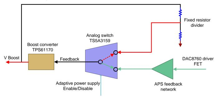
Figure 10. Simplified Block Diagram for Adaptive Power Supply Block
