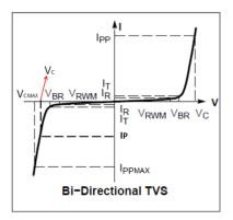
Figure 14. Characteristics of TVS Diode
