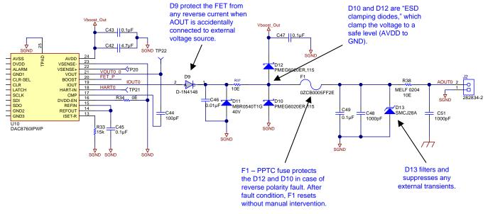
Figure 13. Output Structure of AO Module
