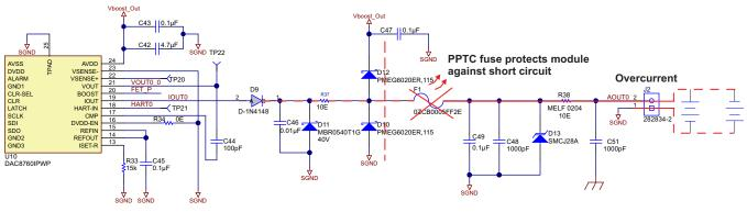
Figure 16. Reverse Voltage Protection
