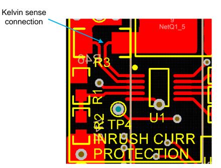
Figure 4. Kelvin Sense Connection for Sense Resistor
