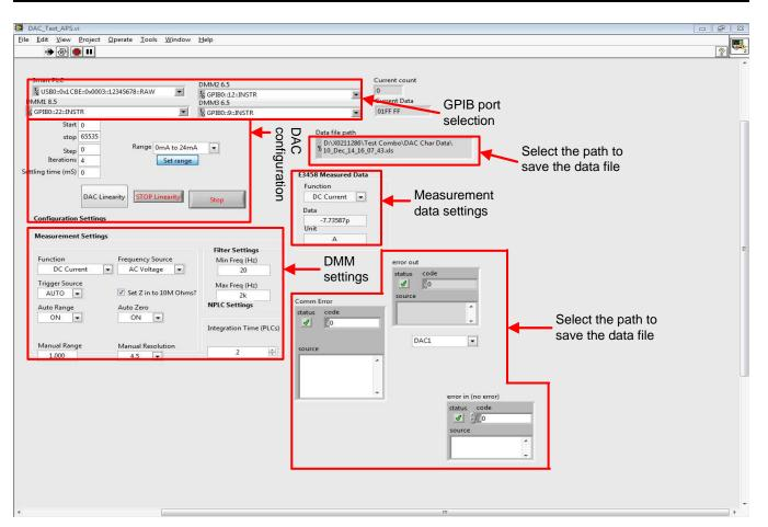
Figure 20. Test GUI Front Panel
