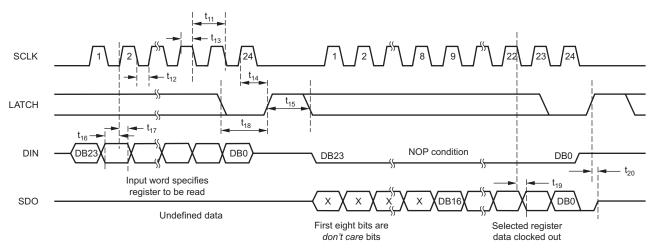
Figure 9. DAC8760 Readback Mode Timing
