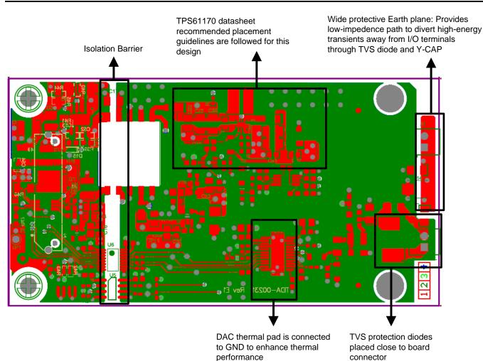
Figure 28. PCB Layout Guidelines
