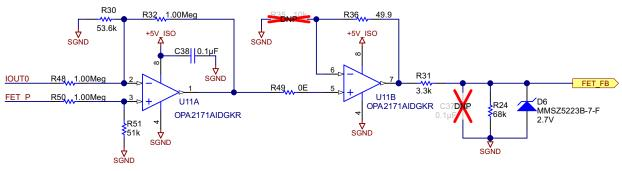
Figure 12. Differential Amplifier and Feedback Control Circuit
