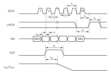
Figure 8. DAC8760 Write Mode Timing
