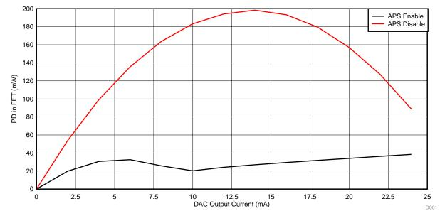
Figure 23. Output Current versus Power Dissipation in FET (Full Range Current Sweep)
