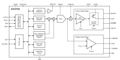
Figure 7. Internal Block Diagram of DAC8760
