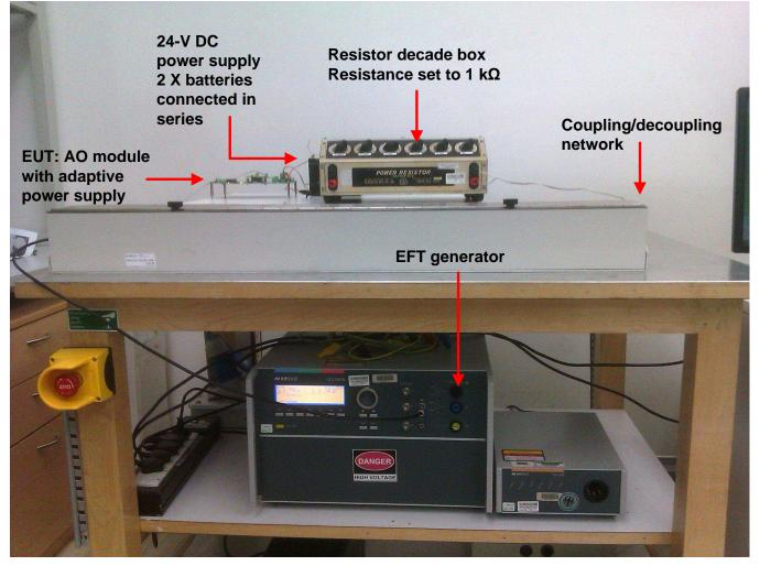
Figure 26. EFT Test Setup
