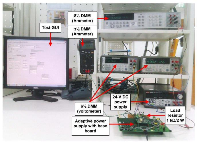
Figure 19. Performance Evaluation Test Setup
