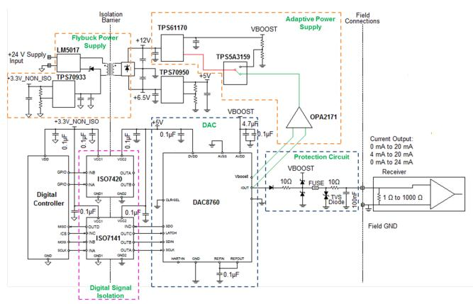
Figure 2. Conceptual Schematic Diagram
