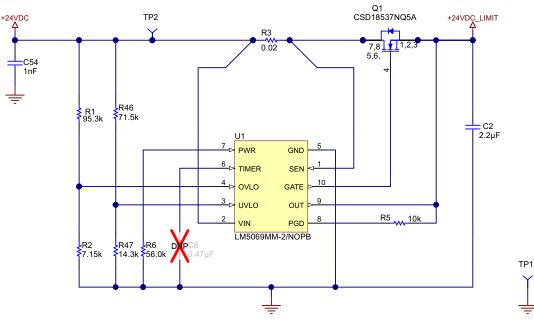
Figure 3. Inrush Current Limit
