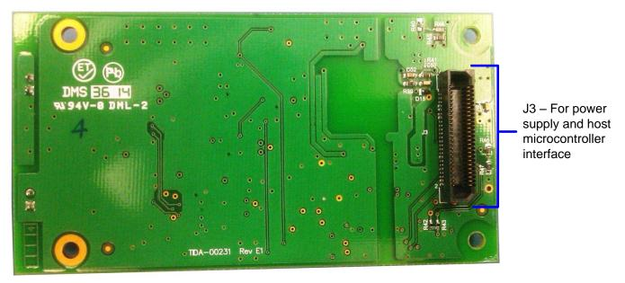
Figure 18. Board Bottom View
