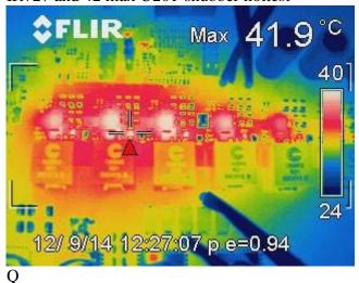
Fan off no other change at 11:18A on lab clock now 11:39 Thermal Image: 12.054Vin 0.9971Vout 325kHz/phase 10.916Ain 120.02Aout 90.9% eff. Fan off 25 minutes stabilized 21-23 deg. C ambient
