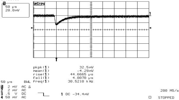
And now from 120A static load to 252A in 10 usec with undershoot also ~25mV  $^{29-Dec-14}$
