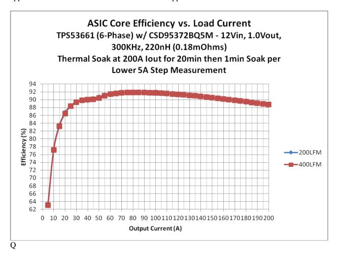
PMP-9738  $\,$  1V  $\,$  200A /  $\,$  255A(peak) 6 phases off 12Vin Test Report (TPS53661 / CSD95372B) Texas Instruments
