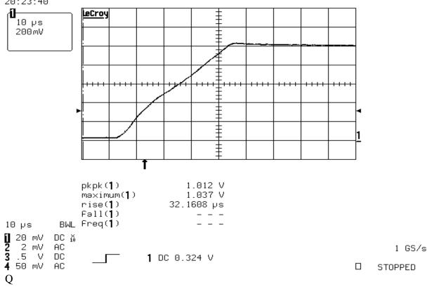
Extreme margining of 1.0 Vout from 80% to 120% of 1.0 V and then back to 80% with constant current load of 120 A: Vin 12.0 V
