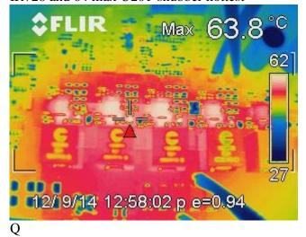
Thermal Image: 12.034Vin 0.9982Vout 321kHz/phase 7.232Ain 80.045Aout 91.8% eff. 5" fan 12.0V 460mA at 5" from UUT 20 minutes stabilized 23 deg. C ambient IR730 and 37 max U201-snubber hottest
