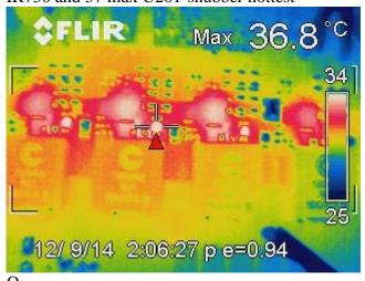
Thermal Image: 12.035Vin 0.9984Vout 318kHz/phase 3.700Ain 40.016Aout 89.7% 5" fan 12.0V 460mA at 5" from UUT 20 minutes stabilized 23 deg. C ambient
