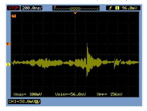
TPS84620: VIN = 12V, VOUT = 5V, IOUT = 3.3A Output Ripple Voltage
