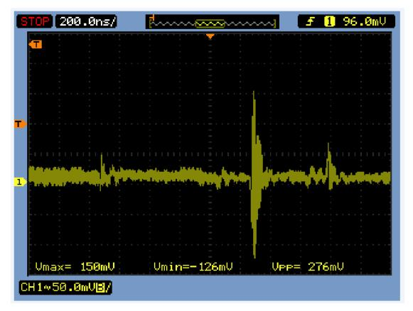
LM3150: VIN = 12V, VOUT = 3.3V, IOUT = 2.5A Output Ripple Voltage
