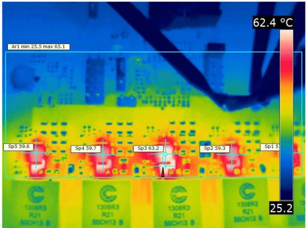
11.9992 Vin, 12.371 Ain, 611.4mVout 200.6A out 25.79 W loss Current senses from the CSD95372Bs: Ref in for all at 1.699 V Iout (pin 1) for each going from left to right in Volts: 1.908; 1.881; 1.895; 1.881; 1.893 Currents in each based upon 5mV/A sense: 41.8A, 36.4A, 39.2A, 36.4A, 38.8A Here, overall variation 5.4A overall variation or 192.6A in all per senses.
