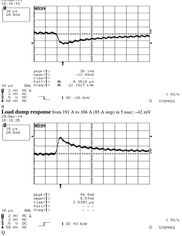
Step load response from 106 A to 176 A (70 A step) in 8 usec: ~30 mV
