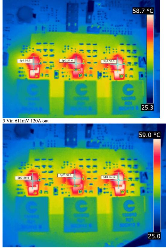
Thermal Images for 3 phase experiment with U200 CSD95373B (cont.) 8 Vin 611mV 120A out
