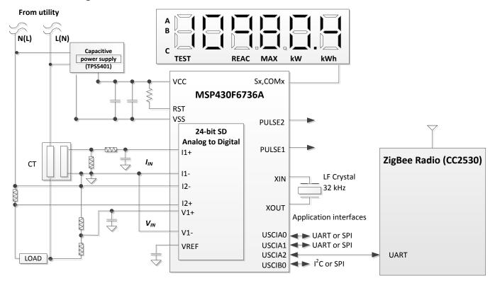
Figure 1. TIDM-1PHMTR-ESD System Block Diagram
