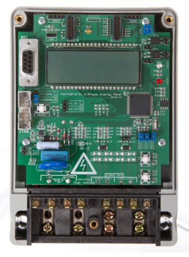
Figure 14. Top View of the Single-Phase Energy Meter EVM
