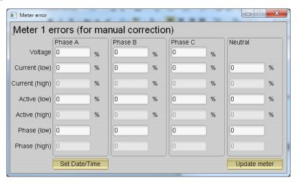
Figure 33. Manual Calibration Window
