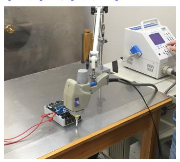
Figure 21. ESD Test Setup
