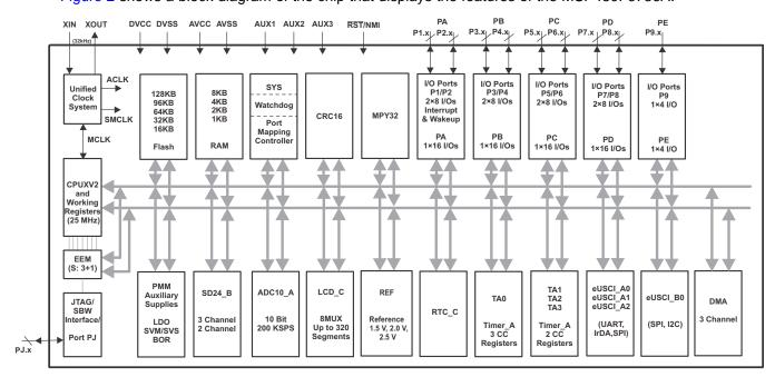
Figure 2 shows a block diagram of the chip that displays the features of the MSP430F6736A.
