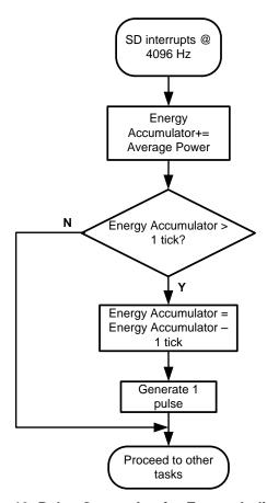
Figure 13. Pulse Generation for Energy Indication
