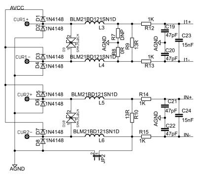
Figure 7. Analog Front End for Current Inputs
