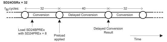
Figure 11. Phase Compensation Using PRELOAD Register
