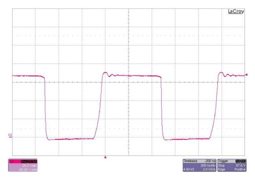
The photo below shows the FET switching voltage (TP5) for an input voltage of 57V and a 0.14A load. The converter has just transitioned to DCM at this load. (20V/DIV, 200nS/DIV)
