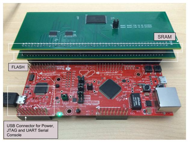
Figure 10. Full Test Assembly (Stacked Flash and SRAM)
