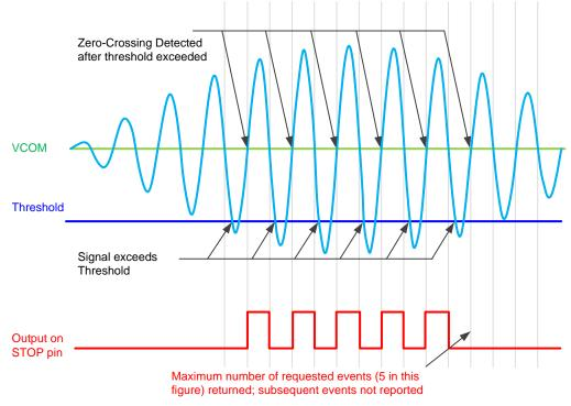
Figure 3. Received Signal to Stop Pulses Conversion
