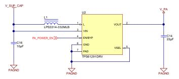
Figure 18. Boost Converter With Super Capacitor (in Part 13)
