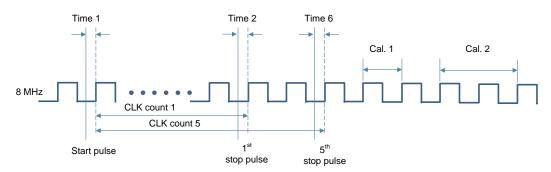
Figure 4. Timing Registers on Five Stop Pulses
