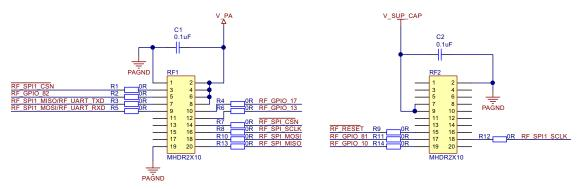
Figure 20. Socket for Connection of Communication Module (Wired or Wireless Type)
