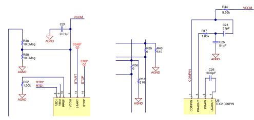
Figure 22. Critical External Passive Circuits of TDC1000
