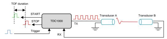
Figure 2. Time of Flight Measurement
