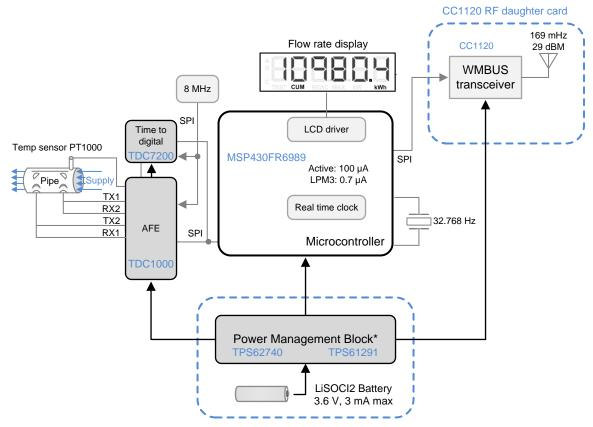
Figure 5. System Block Diagram
