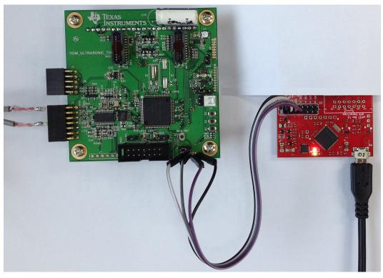
Figure 31. System Setup to Measure of Current Consumption
