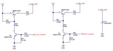
Figure 19. Resistive Charging Circuit for Super Capacitor
