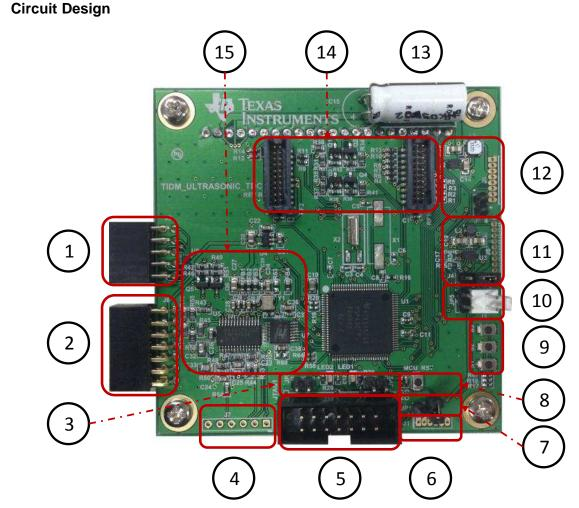
Figure 6. TI Design of Ultrasonic Flow Meter
