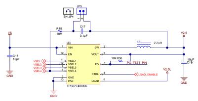
Figure 17. Buck Converter Using TPS62740 to Provide  $V_{cc}$  to the System
