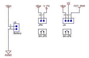
Figure 16. Battery Connector Using 3.6-V Lithium Battery
