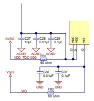
Figure 21. Low-Pass Filters for Power Supplies of TDC1000
