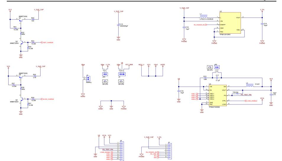
Figure 37. Power Circuit Schematic
