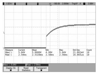
Figure 8. No Capacitor C6; Tau = N/A; Measured T<sub>RISE</sub> = 2.54 ms
