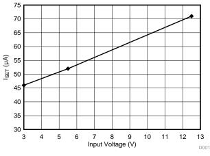
Figure 3. I<sub>SET</sub> versus Input Voltage
