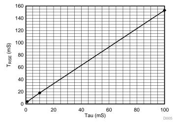
Figure 7. Output Voltage Rise Time (T<sub>RISE</sub>) versus RC Time Constant (Tau)
