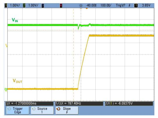
Figure 13.  $V_{OFF}$  from High to Low
