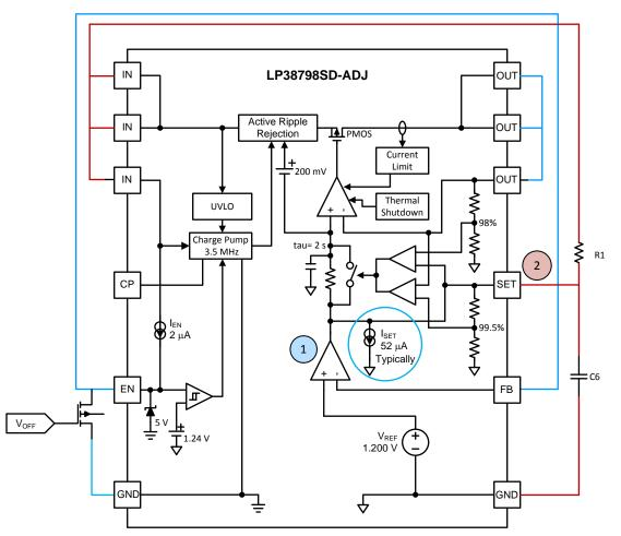
Figure 2. LP38798SD-ADJ Functional Block Diagram
