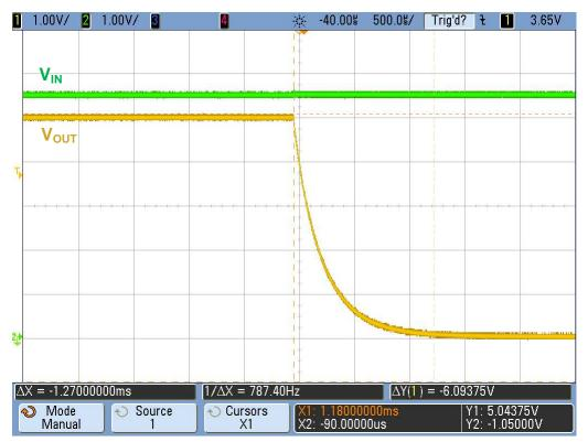
Figure 12. V<sub>OFF</sub> from Low to High
