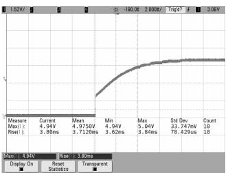
Figure 9. Tau = 1 ms; Measured  $T_{RISE}$  = 3.80 ms
