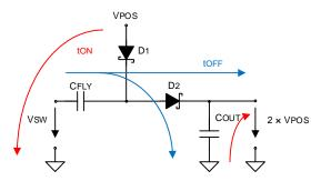
Figure 2. Positive Charge Pump Doubler
