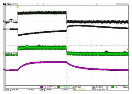
Figure 9 shows the load transient of the charge pumps at a load of 0 A to 10 mA.
