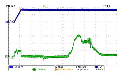
Figure 6. Inrush Current I<sub>IN</sub>
