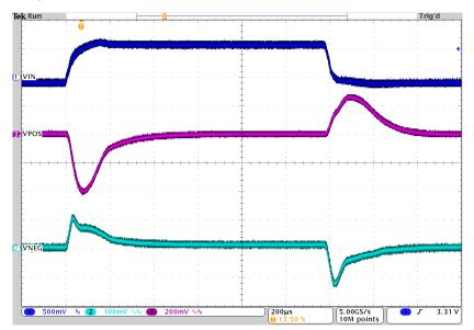
Figure 10.  $V_{\mbox{\tiny POS}}$  and  $V_{\mbox{\tiny NEG}}$  Line Transient Response
