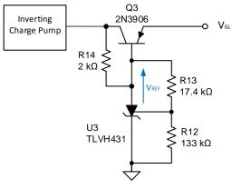
Figure 4. V<sub>GL</sub> Regulator
