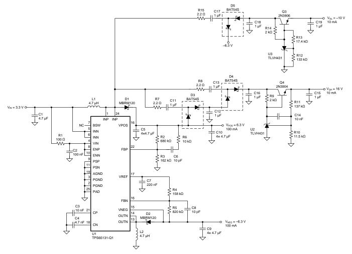
Figure 1. TPS65131-Q1 Circuit Schematic and Charge Pump
