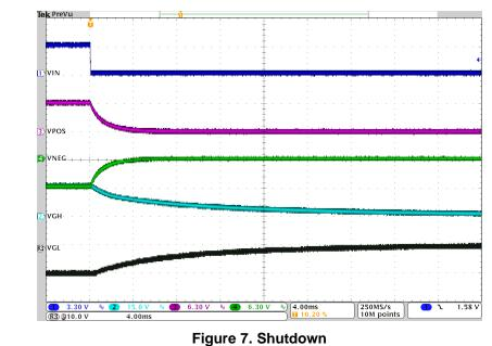
Figure 7 shows the shutdown behavior of the  $V_{POS}$  and  $V_{NEG}$  outputs at a load of 100 mA.
