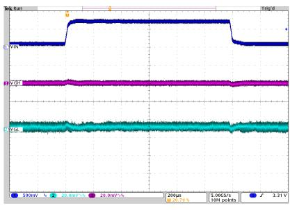
Figure 11. V<sub>GH</sub> and V<sub>GL</sub> Line Transient Response
