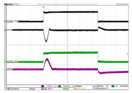
Figure 8.  $V_{POS}$  and  $V_{NEG}$  Load Transient Response (I<sub>OUT</sub> = 0 mA to 100 mA)
