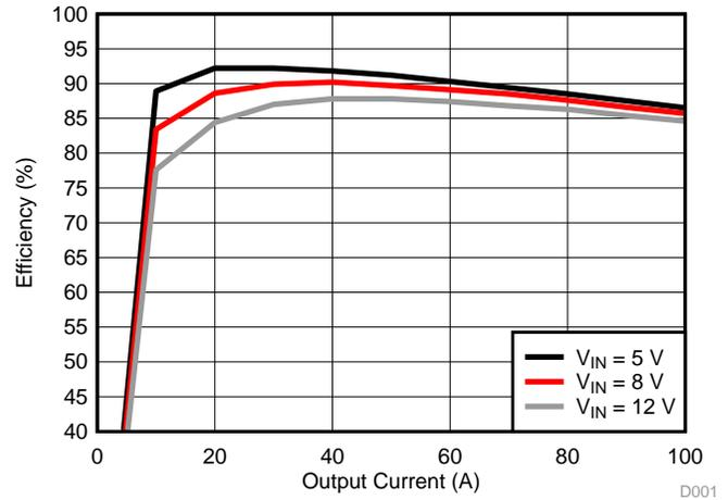
Figure 2. Efficiency, V<sub>OUT</sub> = 1.2 V
