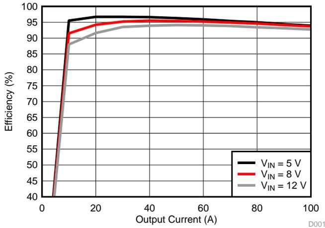
Figure 1. Efficiency, V<sub>OUT</sub> = 3.3 V
