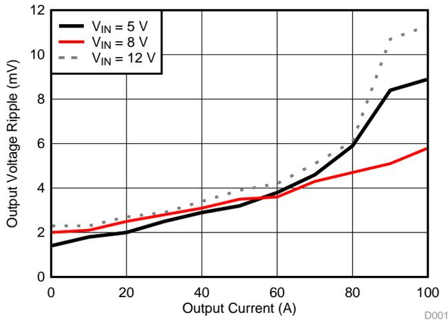
Figure 5. Output Voltage Ripple,  $V_{OUT} = 3.3\text{ V}$
