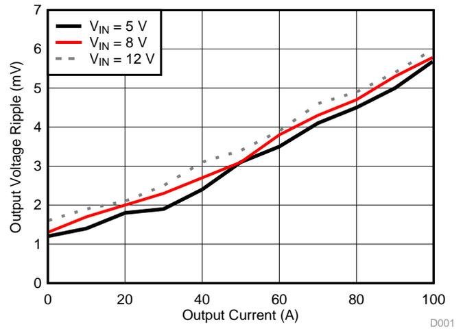
Figure 6. Output Voltage Ripple,  $V_{OUT} = 1.2\text{ V}$
