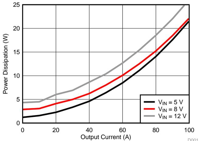
Figure 3. Power Dissipation, V<sub>OUT</sub> = 3.3 V
