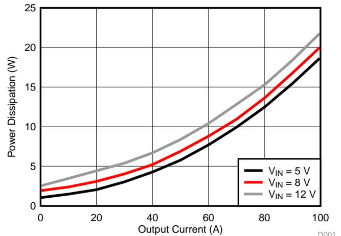
Figure 4. Power Dissipation, V<sub>OUT</sub> = 1.2 V
