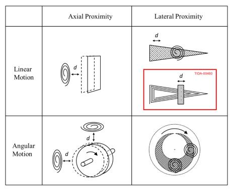
Figure 14. Commonly Used Sensor-Target Configurations
