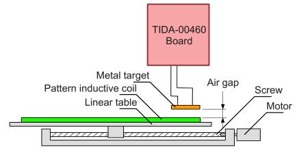
Figure 21. Motorized Linear Table Test Setup
