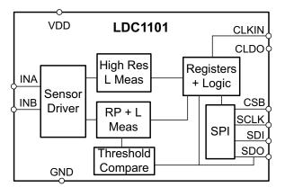
Figure 1. LDC1101 Block Diagram
