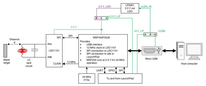
Figure 4. TIDA-00460 Block Diagram
