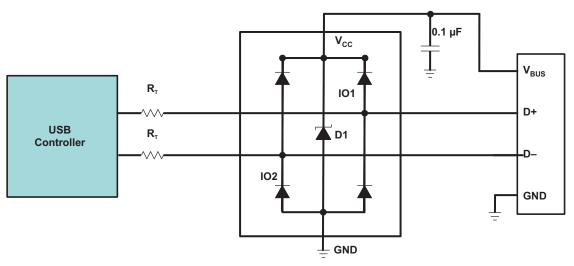
Figure 3. TPD2E001 Block Diagram
