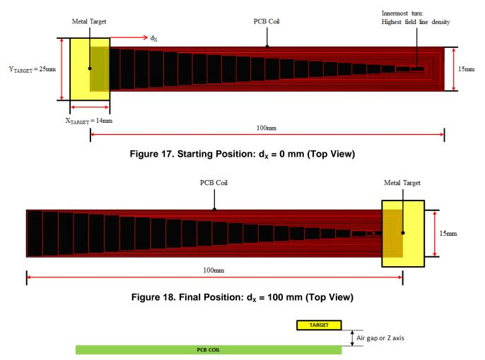
Figure 19. Final Position:  $d_x = 100 \text{ mm}$  (Side View)
