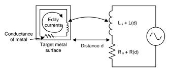
Figure 11. Metal Target Modeled as L and R With Circulating Eddy Currents
