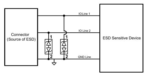
Figure 2. TPD1E10B06 Block Diagram
