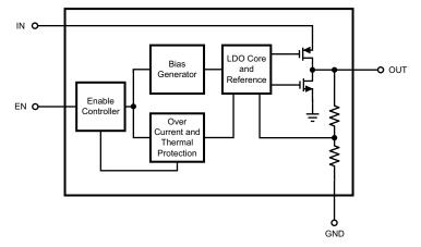
Figure 7. LP5951 Block Diagram
