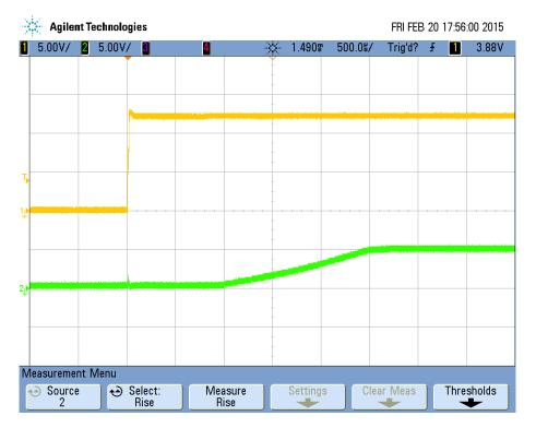
Figure 14 Start up into no load at 12Vin
