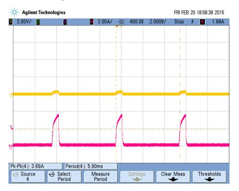
Figure 23 Stay in short circuit at 12Vin
