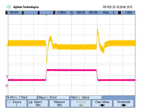
Figure 20 Output load transient 1A to 3A at 12Vin
