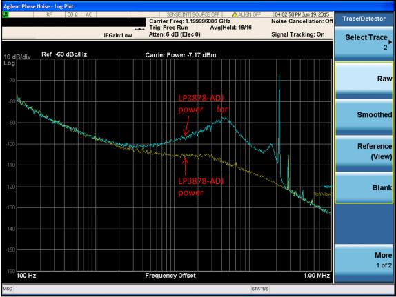
Figure 14 Clock Phase Noise of LP3878-ADJ Power CLK and DCDC Supply Power Core
