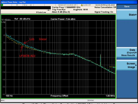
Figure 12 Clock Phase Noise Supplied by LP3878-ADJ and Lab Linear Power
