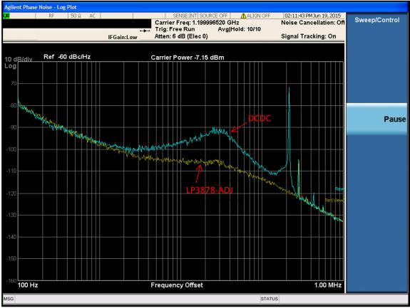
Figure 9 Clock Phase Noise Supplied by LP3878-ADJ and DCDC Switching Supply
