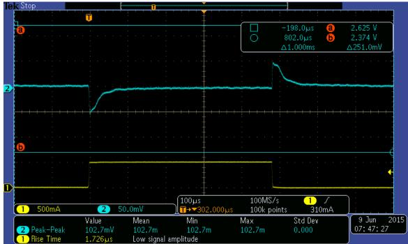
Figure 18 – DCDC3 Load Transient Response @ 25C
