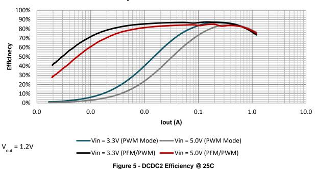
DCDC2 Efficiency vs Load Current @ Ta=25°C
