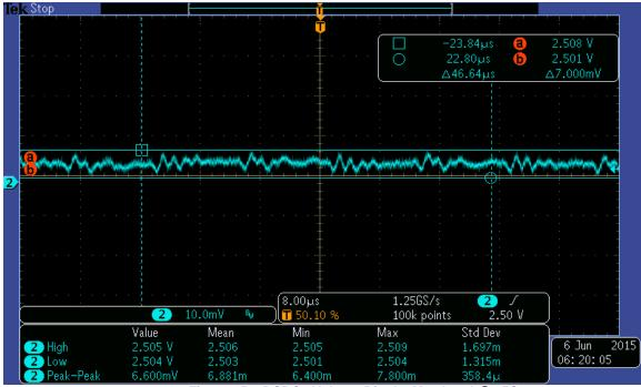
Figure 15 – DCDC3 Voltage Ripple, Max Load @ 25C
