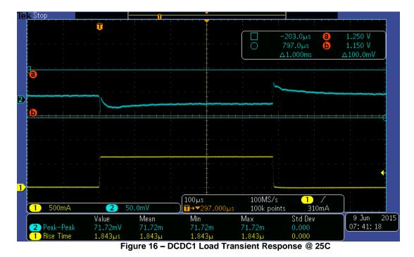
DCDC1 (Vout = 1.2V) – VCCINT Load Step (0mA to 700mA, Rise Time: 15µS; Fall Time: 15µS)
