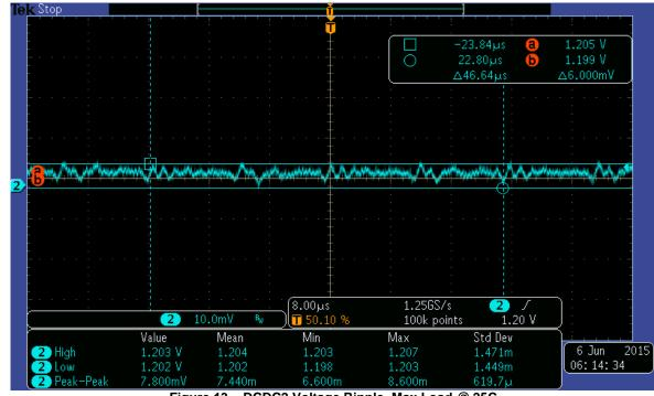
DCDC2 (Vout = 1.2V) - VCCD\_PLL (Max Typical Load)
