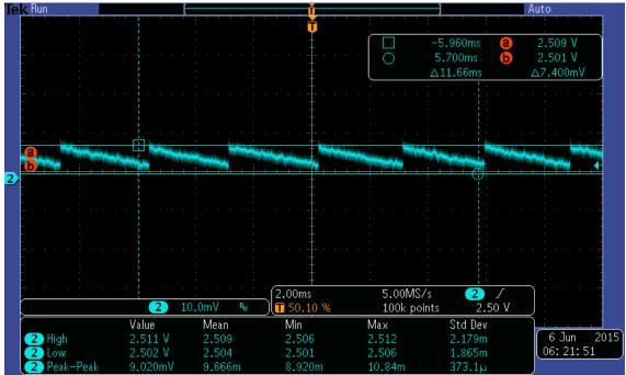
Figure 14 – DCDC3 Voltage Ripple, Light Load @ 25C
