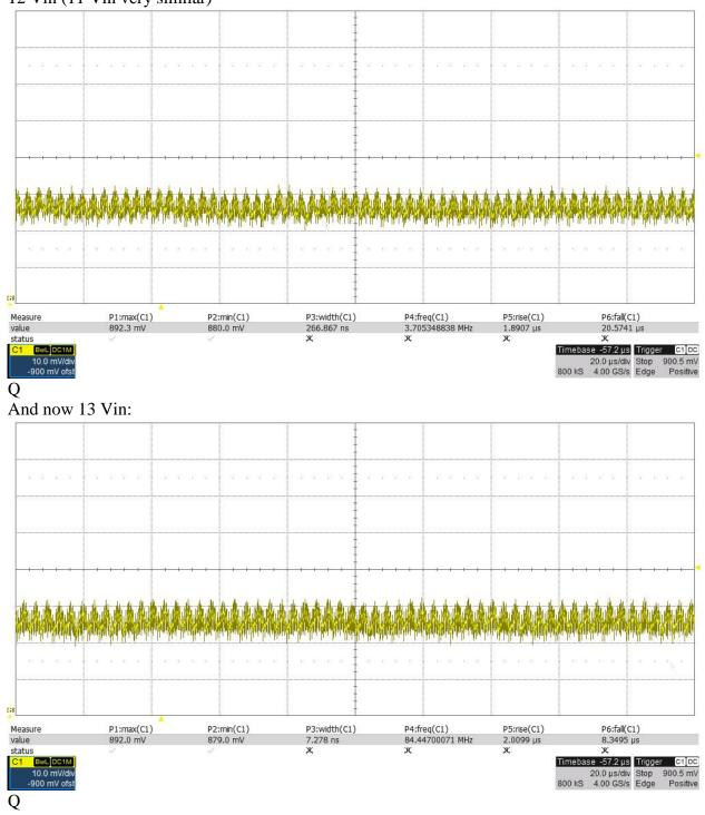
900 mV 300kHz settings: 11.0 VIN quasi constant frequency mode: frequency range 300-308 kHz Vout measured at C19: All 6 phases on
