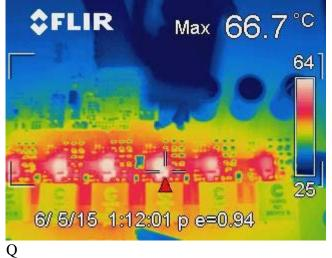
Thermal images: Ambient is 21 degrees Celsius with 1-2 Meters per second airflow: 12Vin 900mV out 240A
