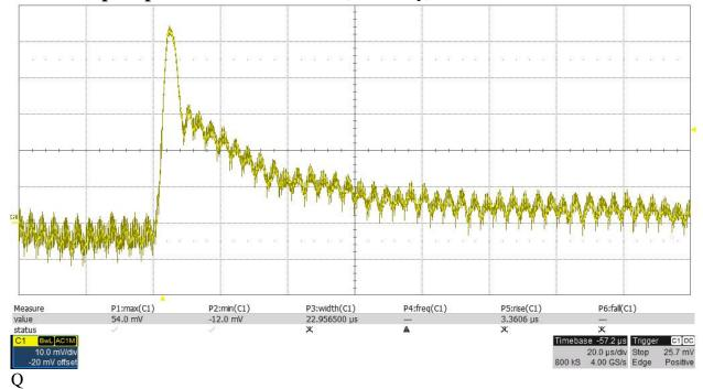
Waveforms across resistors in dynamic load bank used to calculate step load current and speed: There are two resistor paths from Vout; R1 and R2 each 2mOhm and tied to Vout. Hence, the total load step is the sum of both. Here scope ground on Vout side of resistor. First R1 2mOhm: 120 mV in 7 usec or 60 A in 7 usec
