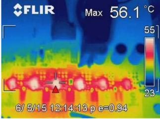
Thermal images: Ambient is 21 degrees Celsius with 1-2 Meters per second airflow: 12Vin 900mV out 220A
