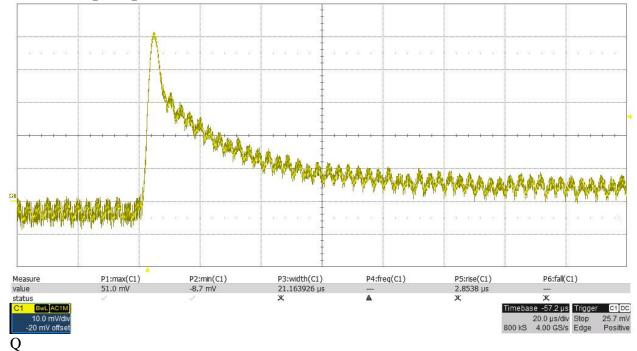
900 mV 300kHz settings: 12.0 VIN Constant on time mode at 60A & quasi constant frequency at 180A: frequency range 288-308 kHz Vout measured at C19: All 6 phases on **Step load response** from 60 A to 180 A (120 A step) in 7 usec: ~31 mV undeshoot
