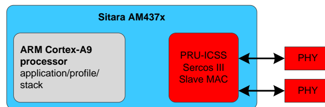
Figure 7. Integrated Sitara Sercos III Slave Solution
