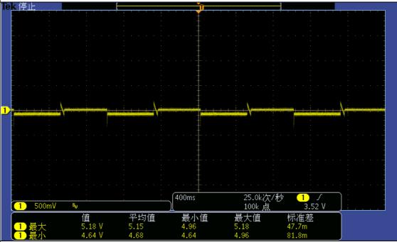
Vin:230Vac test condition: 0%-100% of full load, 0.4A/us, 500ms cycle, 100cm cable Ch1: output voltage
