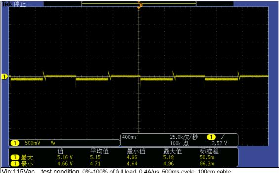
Vin:115Vac test condition: 0%-100% of full load, 0.4A/us, 500ms cycle, 100cm cable Ch1: output voltage
