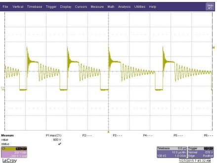
8.2 Voltage at Q1 Drain @ 132V<sub>AC</sub>/60Hz and 24V/1A, 5V/1A (from J4), 5V/0.5A (from J5), 3.3V/1A outputs
