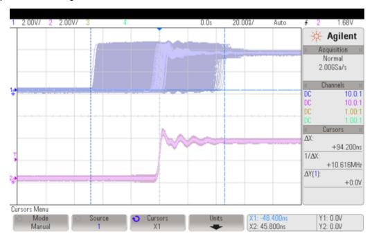
Figure 6. Time Synchronization Jitter in PROFINET IRT Domain
