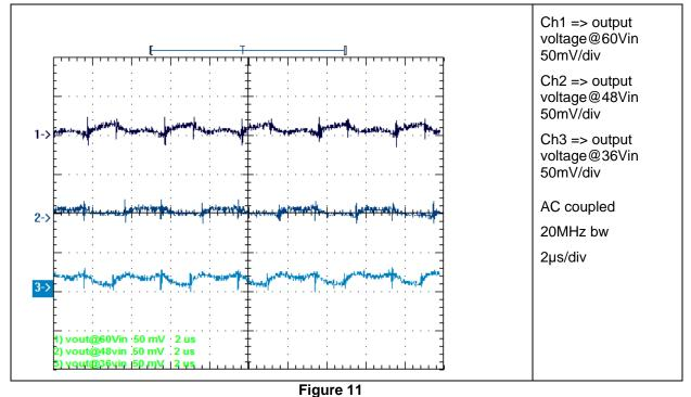
The output voltage ripple voltage is well below specified 100mVpp, here 40mVpp, means only 0.14% for a 28V output.
