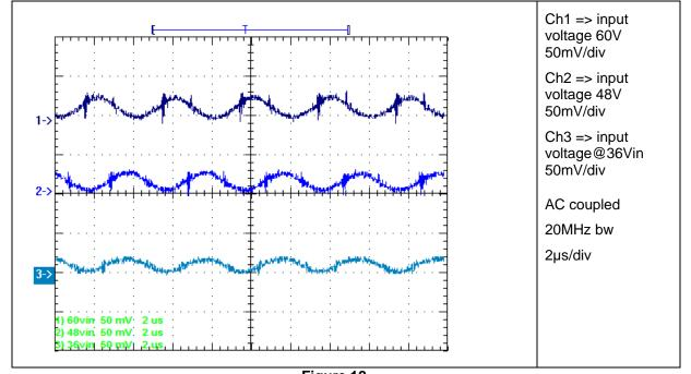
**Figure 12** The input ripple voltage is shown in Figure 13 (measured near C9).
