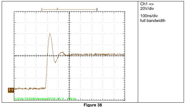
RF noise and overshoot could be reduced simply by adding 470pF (E6) / 33 Ohms (E6) or similar.
