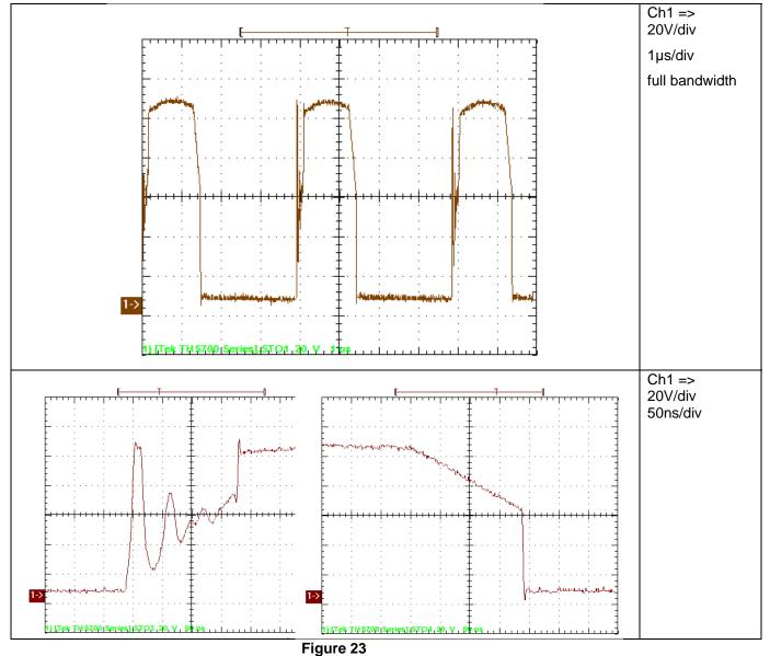
Delay resistor RT of 2.2kOhm offers a shiny drain waveform – but less QR switching and less efficiency; screenshots are taken w/ RT of 16kOhm. Placing 2k55 to 16k in parallel and switching 2k55 shows the difference; 2k2 means hard switching.
