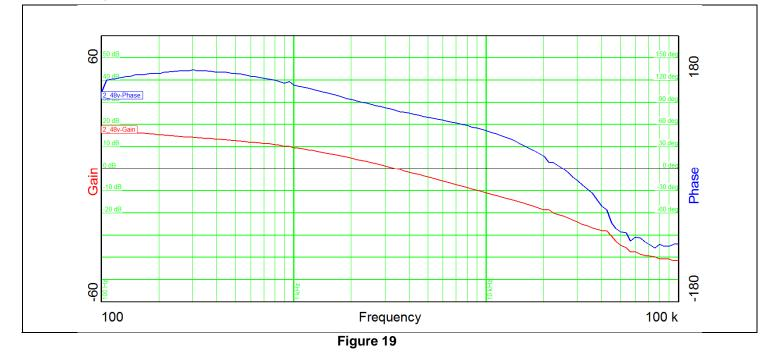
Figure 20 shows the loop response. 2A-load applied. The input voltage was set to 48V (resistor load).
