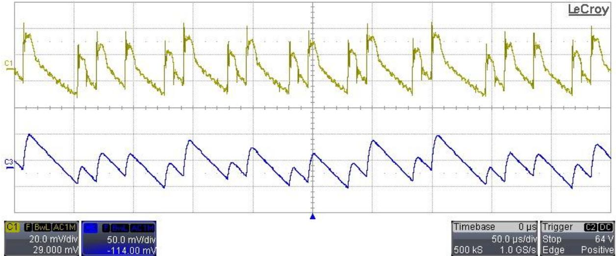
**Ch1: 3.3Vout (20mV/div, 20MHz BWL, AC coupling, 50usec/div)**
