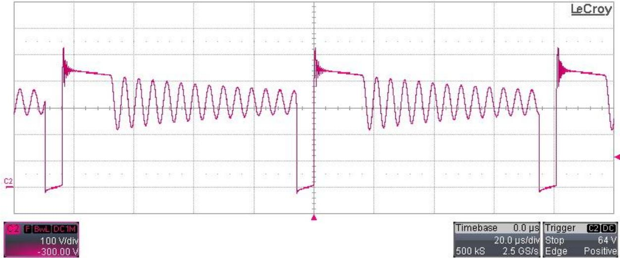
**Ch1: Pin 8 of U1 (100V/div, 20usec/div, 200MHz BWL), 389Vdc\_in**
