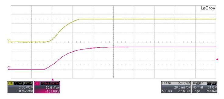
Ch1: Vout (2V/div, 20MHz BWL, 20msec/div) Ch2: Vin (50V/div, 20MHz BWL) No load condition, Vin=127Vdc:
