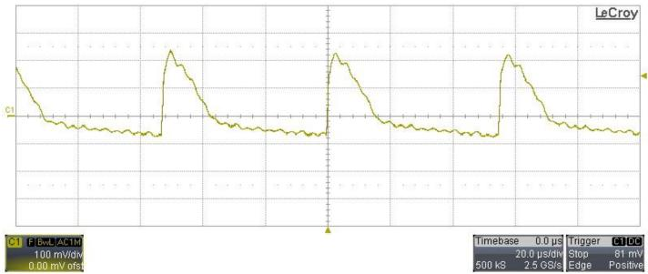
Ch1: Vout (100mV/div, 20MHz BWL, AC coupling, 20usec/div) Vin = 127Vdc
