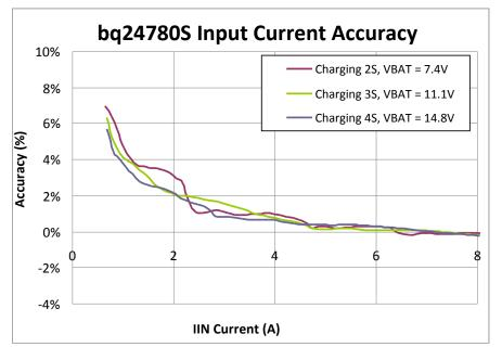
Figure 6. TIDA-00657 Input Current Accuracy
