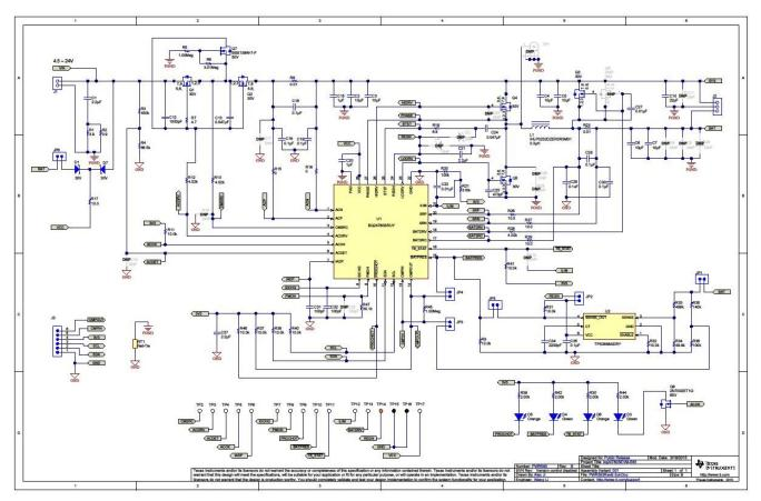
Figure 2. bq24780S Application Circuit
