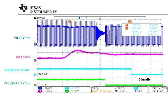
Vin=20V, VBAT = 13.3V, IIN = 2048mA, ICRIT threshold = 150%
