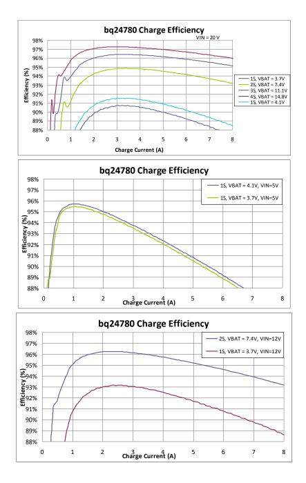
Figure 3. TIDA-00657 Charging Efficiency
