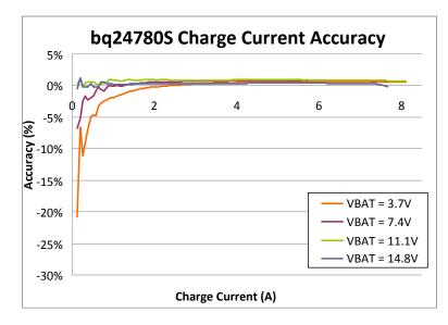
Figure 5. TIDA-00657 Charge Current Accuracy
