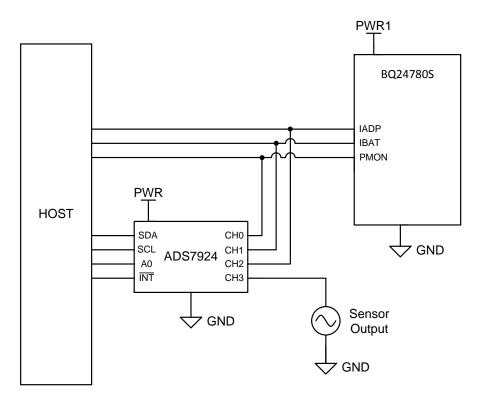
Figure 9. Block Diagram: Autonomous Monitoring Application using ADS7924
