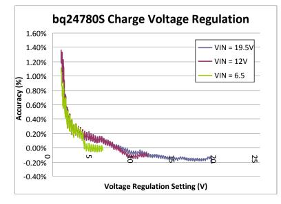
Figure 4 shows the bq24780S charge voltage accuracy across at 25°C
