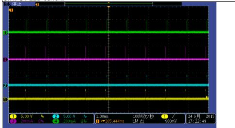
Vin:110Vac lo: LED Lamp load Ch1: DIM\_B1 voltage, Duty=1% Ch2: DIM\_R2 voltage, Duty=1%
