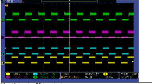
Vin:110Vac Io: LED Lamp load Ch1: DIM\_B1 voltage, Duty=50% Ch2: DIM\_R2 voltage, Duty=50%
