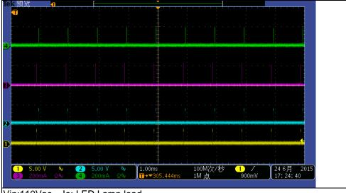
Vin:110Vac lo: LED Lamp load Ch1: DIM\_G2 voltage, Duty=1% Ch2: DIM\_B2 voltage, Duty=1%
