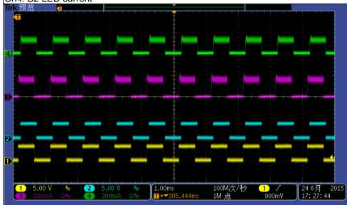
Vin:110Vac Io: LED Lamp load Ch1: DIM\_G2 voltage, Duty=50% Ch2: DIM\_B2 voltage, Duty=50%
