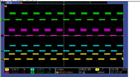
Vin:110Vac Io: LED Lamp load Ch1: DIM\_R1 voltage, Duty=50% Ch2: DIM\_G1 voltage, Duty=50%
