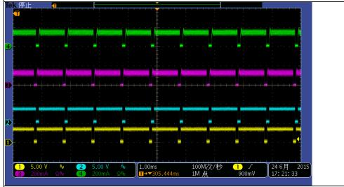
Vin:110Vac lo: LED Lamp load Ch1: DIM\_B1 voltage, Duty=90% Ch2: DIM\_R2 voltage, Duty=90%
