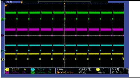
Vin:110Vac Io: LED Lamp load Ch1: DIM\_R1 voltage, Duty=90% Ch2: DIM\_G1 voltage, Duty=90%
