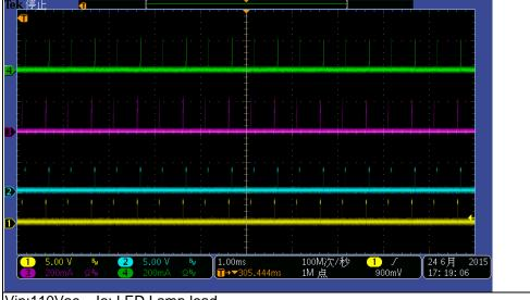
Vin:110Vac lo: LED Lamp load Ch1: DIM\_R1 voltage, Duty=1% Ch2: DIM\_G1 voltage, Duty=1%
