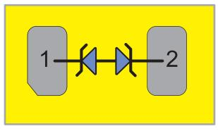
Figure 7. Block Diagram of TPD1E10B06
