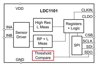
Figure 17. LDC1101 Block Diagram
