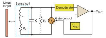
Figure 12. Oscillation Amplitude Regulation
