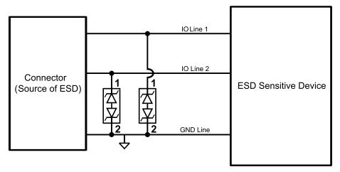
Figure 1. Functional Diagram of TPD1E10B06
