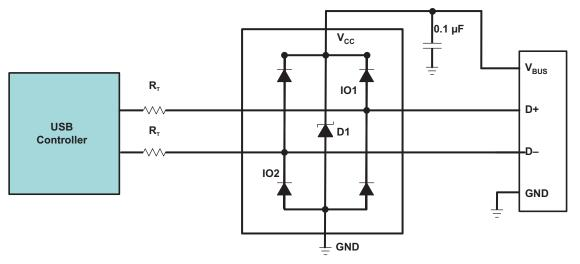
Figure 2. Functional Diagram of TPD2E001
