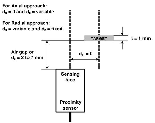
Figure 21. Axial Position Sensing
