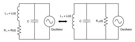
Figure 11. Series and Parallel LC Tank Circuits Connected With Oscillator
