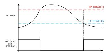
Figure 20. INTB/SDO Output Value for R<sub>P</sub> Comparator With Hysteresis (INTB\_FUNC = b00'0010)
