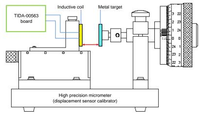
Figure 22. TIDA-00563 Test Setup
