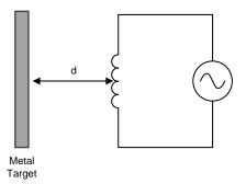
Figure 9. Inductor With Metal Target
