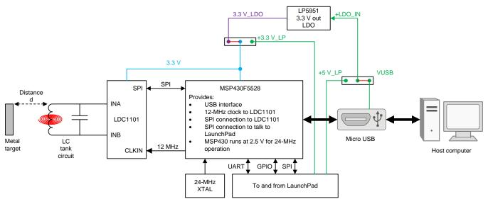
Figure 3. Block Diagram of TIDA-00563
