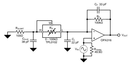
Figure 4: Detailed Programmable Gain Amplifier Circuit Schematic
