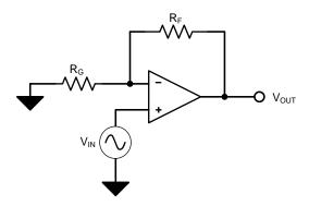
Figure 2: Non-Inverting Amplifier Circuit
