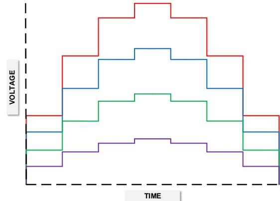
**Figure 2.** 1/4 Step Current Regulation Scaled by TRQ Percentage
