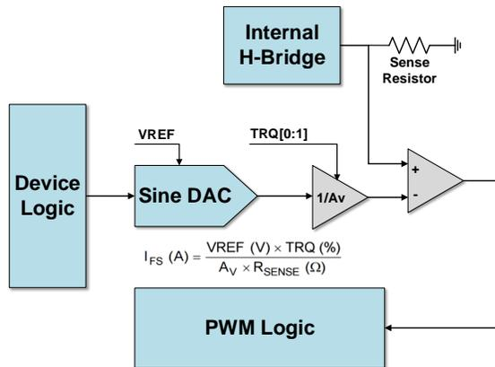
**Figure 1.** Single Phase Current Regulation Control Scheme
