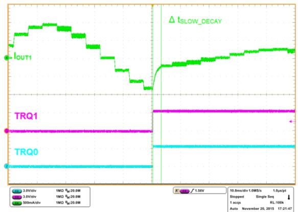
Figure 7. Slow / Fast Decay 100% - 25% Torque Change
