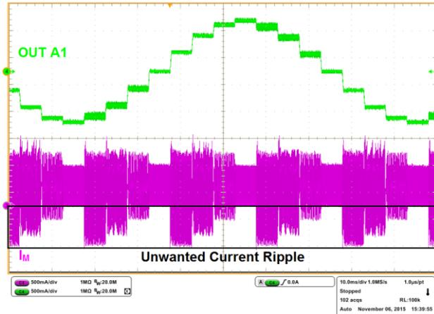
**Figure 3.** Supply Current Ripple Using Fast / Slow Decay
