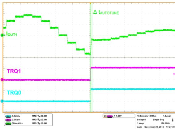
Figure 6. AutoTune 100% - 25% Torque Change
