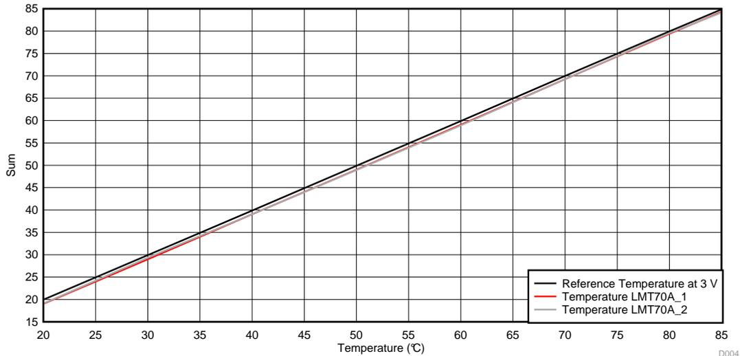
Figure 12. Two LMT70A Sensors in Precision Temperature Oil Bath
