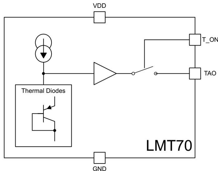
**Figure 1. LMT70A Block Diagram**
