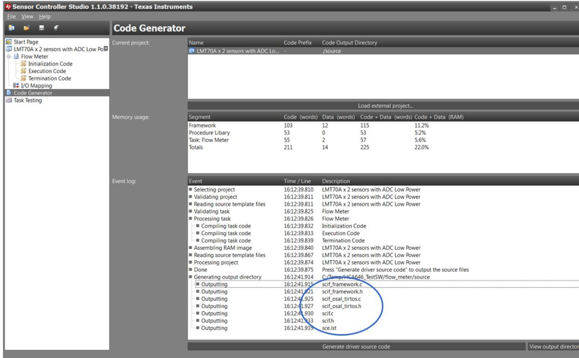
Figure 8. Sensor Controller Output Files Included in IAR Project
