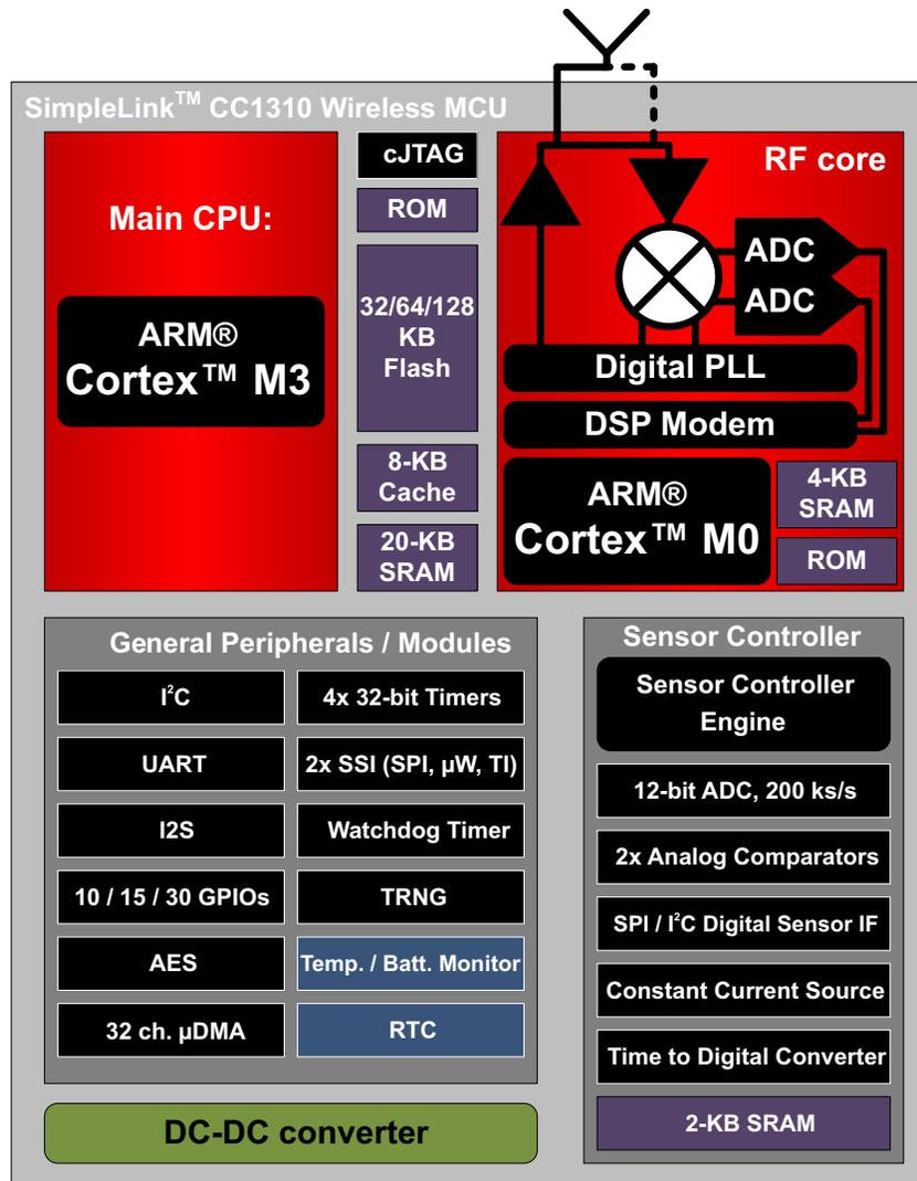
**Figure 2. CC1310 Functional Block Diagram**
