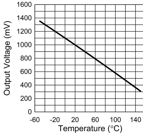
**Figure 4. LMT70 Output Transfer Function**
