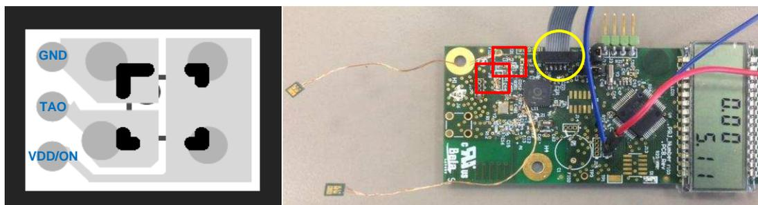
**Figure 5. Small PCB Layout for LMT70 (Left) and Two PCBs Soldered to TIDA-00646 (Right)**
