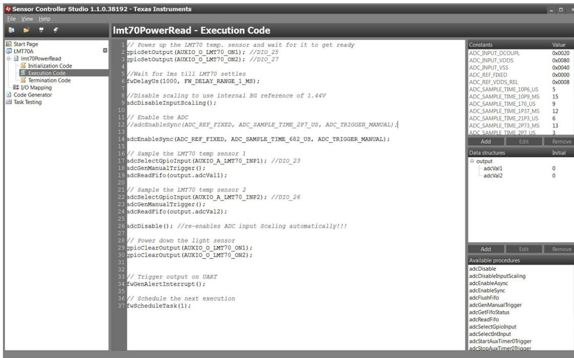
**Figure 7. Sensor Controller Project for CC1310 and LMT70A Readout of Each Sensor**
