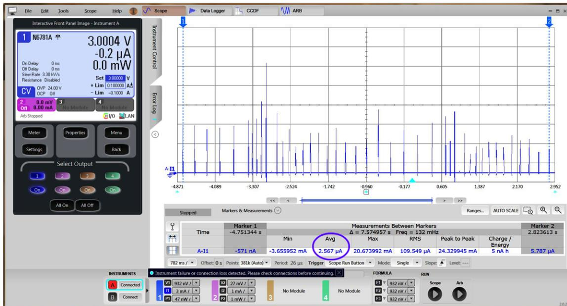
Figure 13. Two LMT70A Sensors Read Out By CC1310 Every Four Seconds
