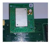
The CC2530-CC2592EM can also be plugged into the SmartRF05 battery boards for standalone applications.
