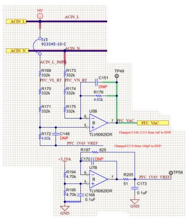
Figure 2-2. Input AC Voltage Sensing Circuit
