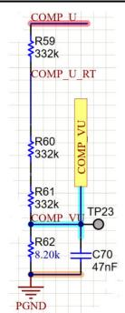
Figure 2-35. Motor Voltage Sensing Circuit
