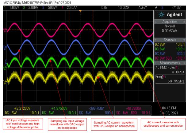
Figure 3-26. Build Level 4: Voltage and Current of PFC
