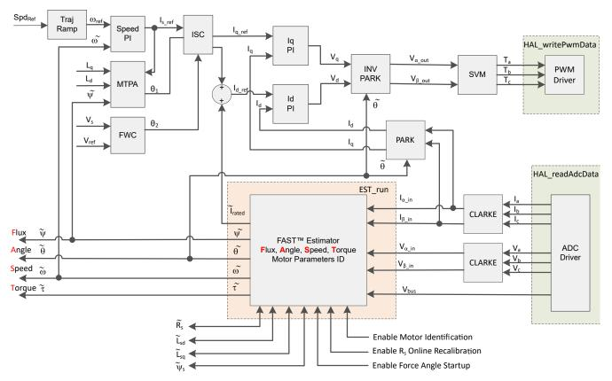
Figure 2-15. Sensorless FOC of Compressor PMSM using FAST with FWC and MTPA
