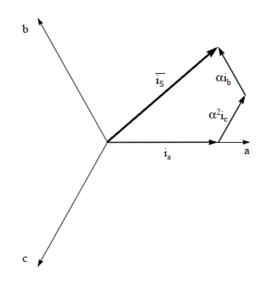
Figure 2-7. Stator Current Space Vector and its Component in (a,b,c) Frame
