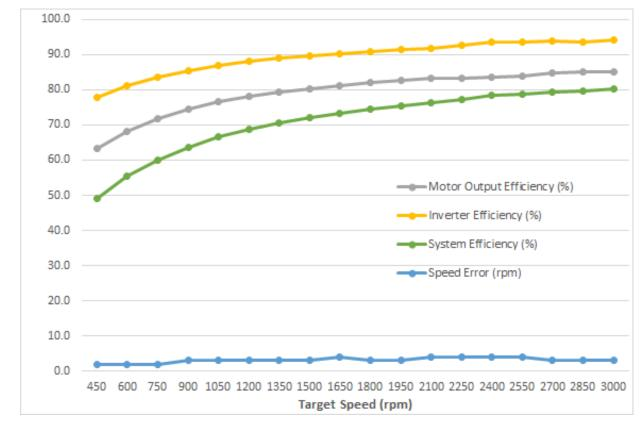
Figure 3-35. Fan Motor Output and Inverter Efficiency at Different Speed with Constant Load
