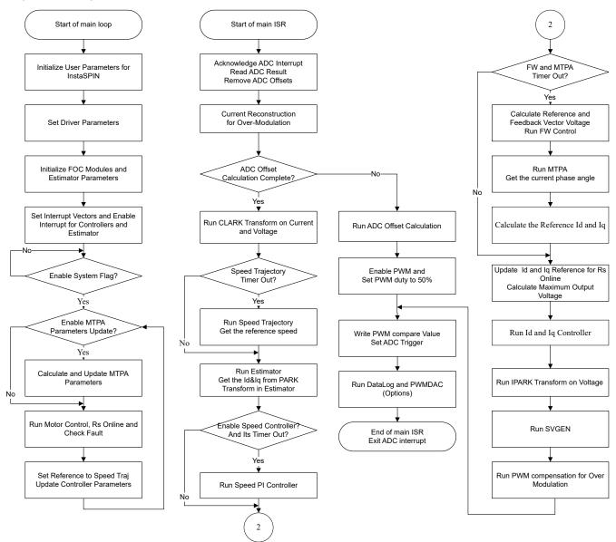
Figure 2-26 is the flowchart that shows the steps required to run InstaSPIN-FOC with FW and MPTA in the main loop and interrupt.
