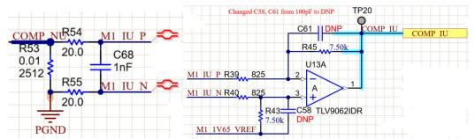
Figure 2-32. Motor Current Sensing Circuit with Three-Shunt
