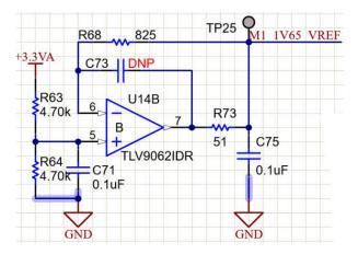
Figure 2-31. 1.65-V Reference from 3.3-V Input Circuit
