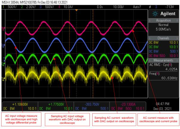
Figure 3-22. Build Level 3: AC Voltage, Current of PFC
