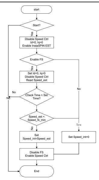
Figure 2-30. Flying Start Module Program Flowchart
