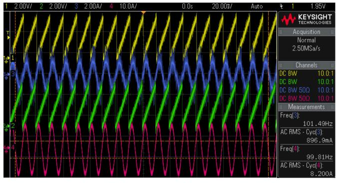
Figure 3-33. Phase Current and Rotor Angle of Fan and Compressor Motors
