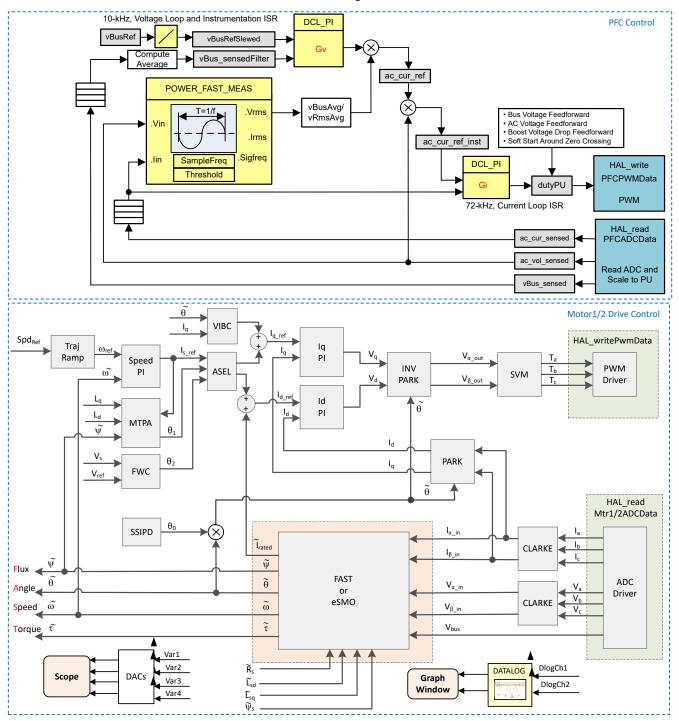
Figure 3-23. Control Software Block Diagram: Build Level 4 – Speed and Current Close Loop Control
