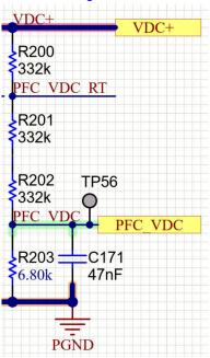
Figure 2-3. DC Bus Voltage Sensing Circuit
