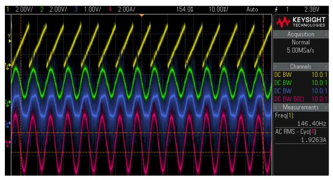
Figure 3-29. Phase Current and Voltage Waveforms of Fan Motor at 150Hz
