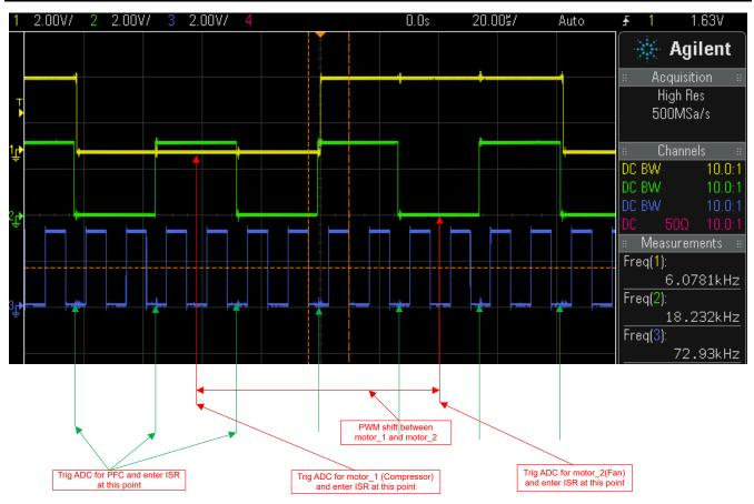
Figure 3-13. Build Level 1: Dual Motor and PFC PWM Output
