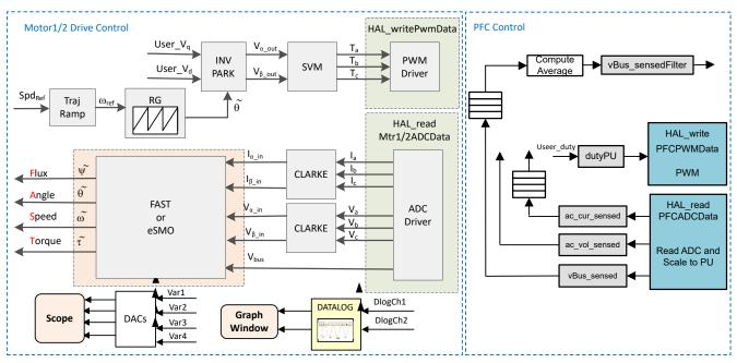
Figure 3-15. Control Software Block Diagram: Build Level 2 – Open Loop Control
