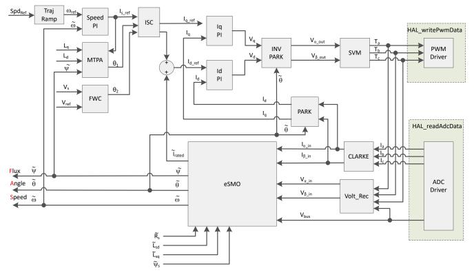
Figure 2-13. Sensorless FOC of Compressor PMSM using eSMO with FWC and MTPA
