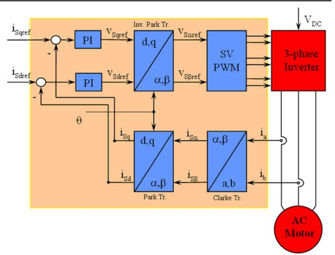
Figure 2-10. Basic Scheme of FOC for AC Motor
