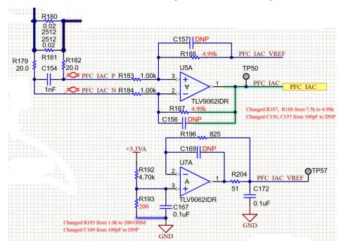
Figure 2-4. PFC Bus Current Sensing Circuit
