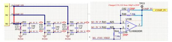
Figure 2-33. Motor Current Sensing Circuit with Single-Shunt
