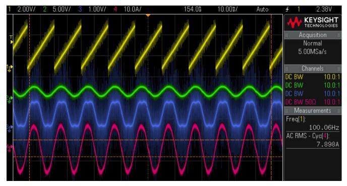
Figure 3-30. Phase Current and Voltage Waveforms of Compressor Motor at 100Hz
