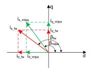
Figure 2-25. Current Phasor Diagram of an IPMSM During FW and MTPA
