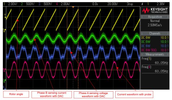
Figure 3-21. Build Level 3: Rotor Angle, Phase Current of Motor
