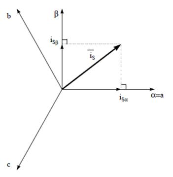
Figure 2-8. Stator Current Space Vector in the Stationary Reference Frame
