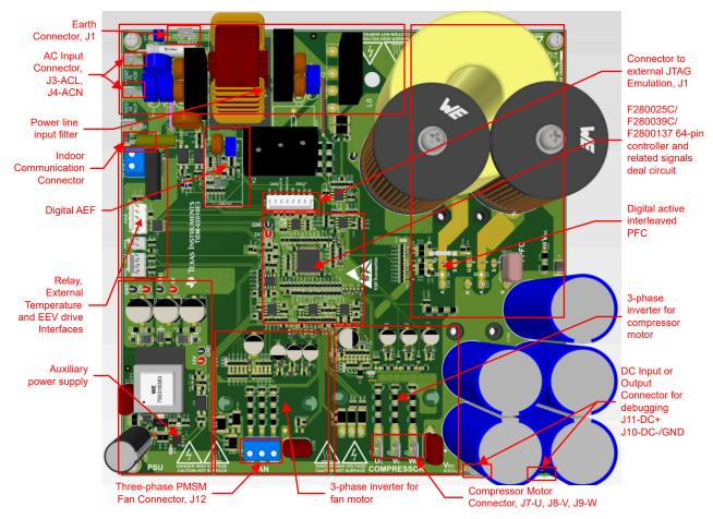
Figure 3-2. The Layout of Dual Motor Control with PFC Reference Design Board
