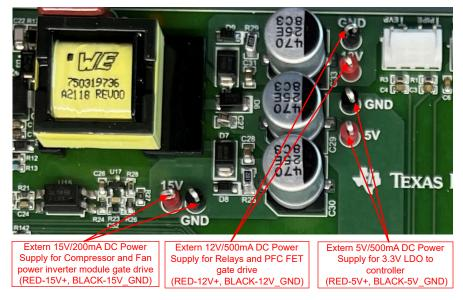
Figure 3-10. Connect the External DC Power Supply to Verify the Hardware
