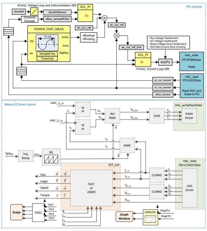
Figure 3-19. Control Software Block Diagram: Build Level 3 – Current Close Loop Control
