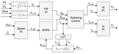
Figure 2-24. Block Diagram of Field-Weakening and Maximum Torque per Ampere Control
