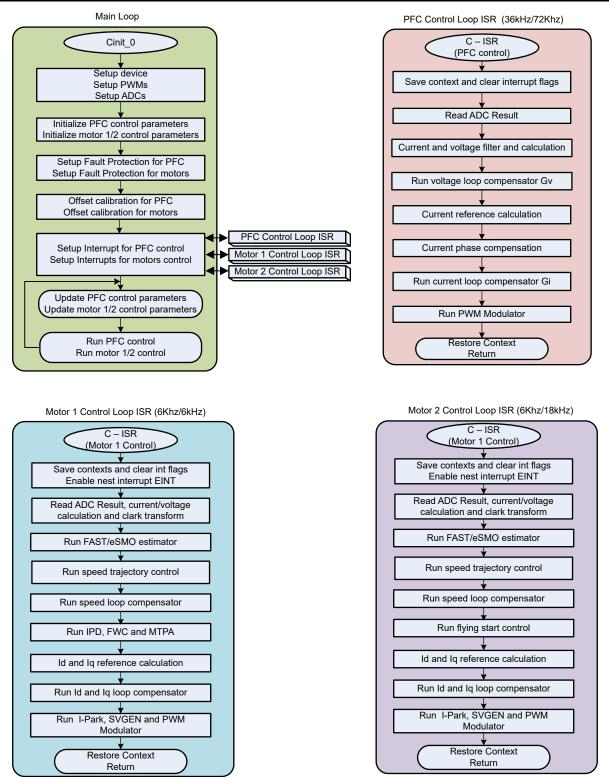
Figure 3-8. Project Flow Diagram of the Firmware
