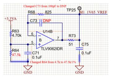
Figure 2-34. DC Offset Reference from 3.3-V Input Circuit
