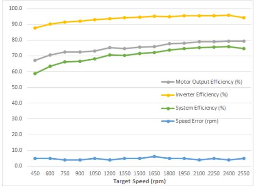
Figure 3-37. Compressor Motor Output and Inverter Efficiency at Different Speed with Constant Load
