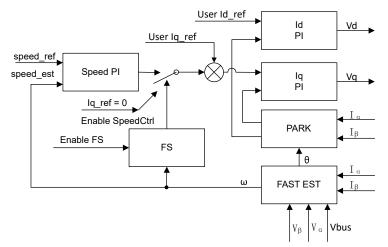
Figure 2-29. Flying Start Control Block Diagram
