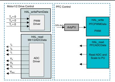
Figure 3-9. Control Software Block Diagram: Build Level 1 – Offset Validation
