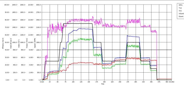
Figure 3-28. Compressor Motor Output Power and Efficiency at Various Speed and Load
