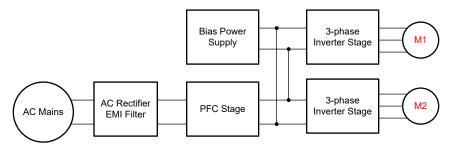
Figure 3-1. Hardware Board Block Diagram of TIDM-02010
