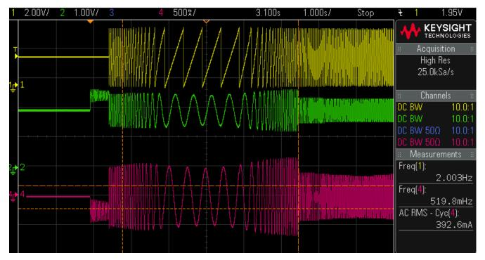
Figure 3-31. Phase Current and Rotor Angle of Fan Motor without Flying Start
