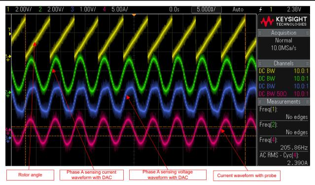
Figure 3-25. Build Level 4: Rotor Angle, Phase Current of Motor
