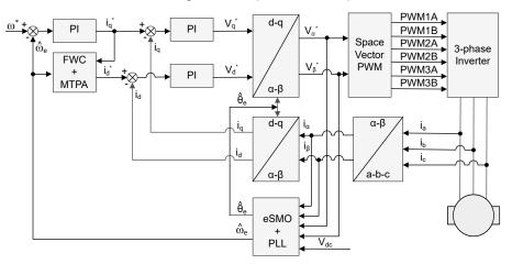
Figure 2-16. Sensorless FOC Structure of an IPMSM System
