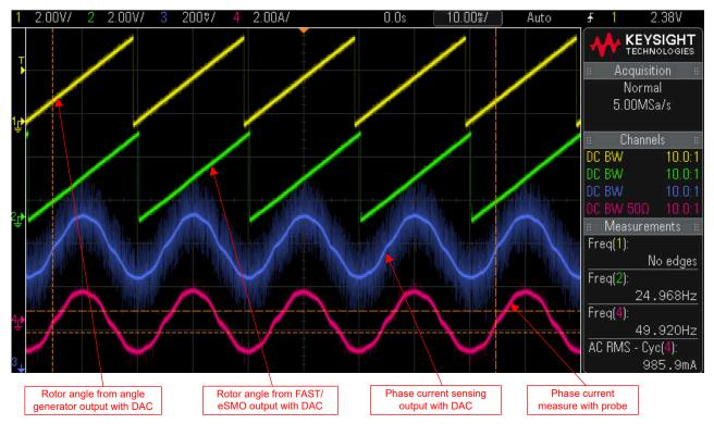
Figure 3-17. Build Level 2: Rotor Angle, Phase Current of Motor
