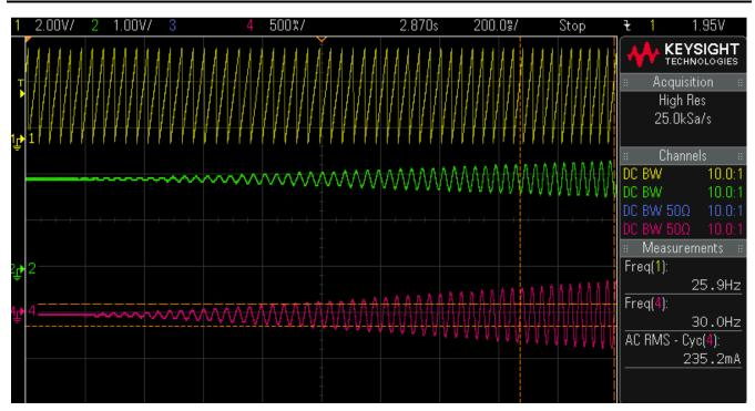
Figure 3-32. Phase Current and Rotor Angle of Fan Motor with Flying Start
