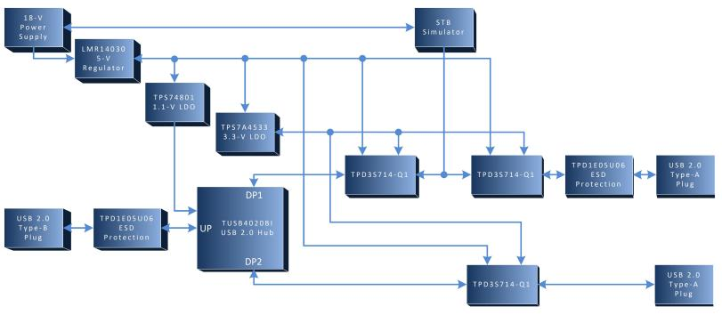
Figure 1. TIDA-00845 Functional Block Diagram
