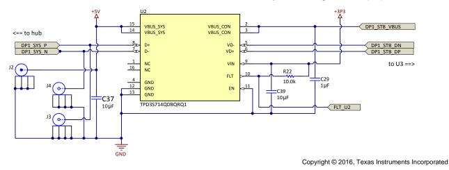
Figure 2. TPD3S714-Q1 Protecting Hub from STB on DP1
