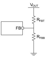
Figure 8. Output Voltage Setting
