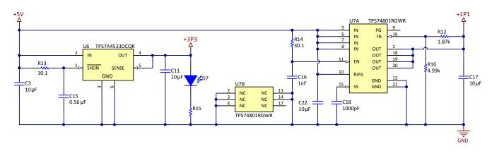
Figure 25. VDD33 and VDD Power Rails
