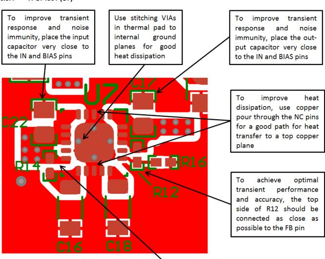
To minimize the voltage drop on the BIAS pin during transient conditions, the trace length between the BIAS pin and the  $V_{\rm IN}$  node should be minimized. This also improves the turn-on response
