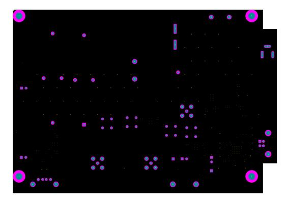
Figure 35. Bottom Solder Mask
