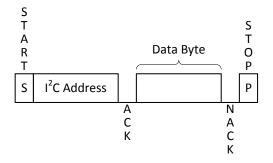
Figure 7. I<sup>2</sup>C Current Address Read Timing Diagram
