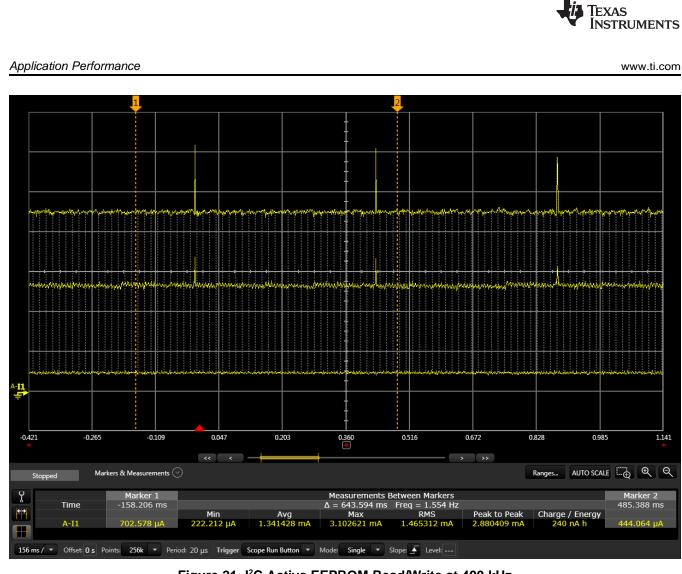
Figure 21. I<sup>2</sup>C Active EEPROM Read/Write at 400 kHz
