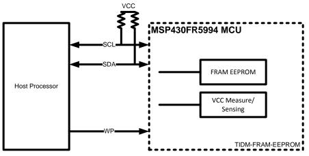
Figure 3. EEPROM I<sup>2</sup>C Interface Block Diagram
