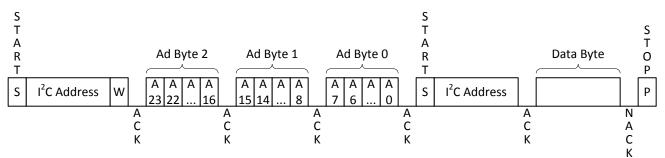
Figure 8. I<sup>2</sup>C Random Read Timing Diagram
