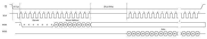
Figure 13. SPI Sensor Data Read Timing Diagram
