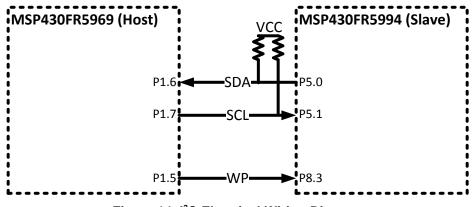
Figure 14. I<sup>2</sup>C Electrical Wiring Diagram
