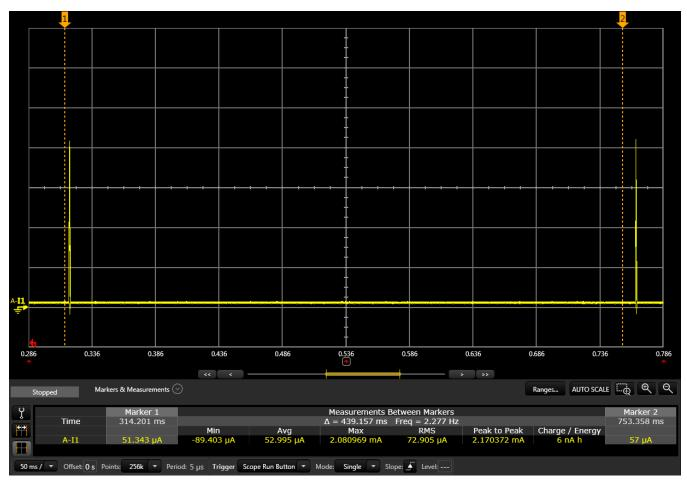
Figure 20. I<sup>2</sup>C Standby Current Profile
