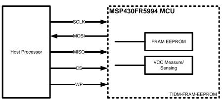
Figure 2. EEPROM SPI Block Diagram
