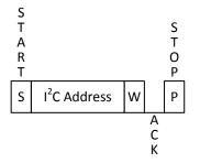
Figure 6. I<sup>2</sup>C Acknowledge Polling Timing Diagram
