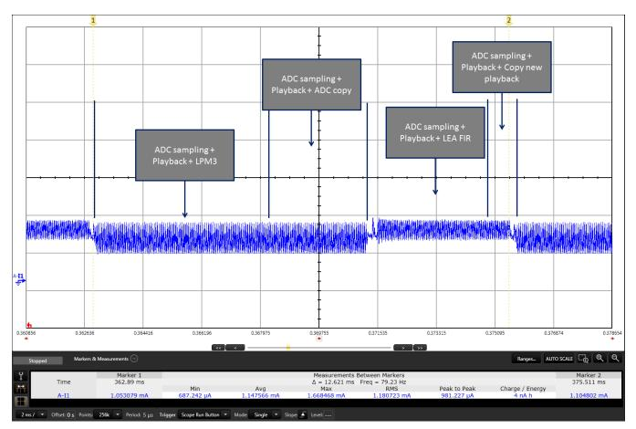
Figure 17. FIR Average Current Without Audio BoosterPack and Graphics LCD
