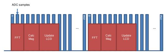
Figure 3. Generic Timing Diagram for FFT Operation
