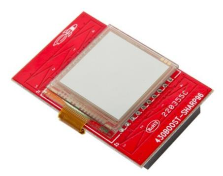
Figure 8. 430BOOST-SHARP96 Graphics LCD BoosterPack
