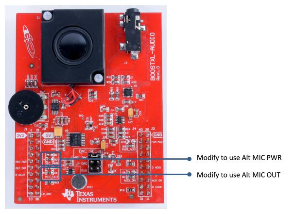
Figure 7. BOOSTXL-AUDIO BoosterPack Required Modification
