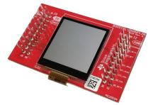
Figure 9. BOOSXL-SHARP128 Graphics LCD BoosterPack
