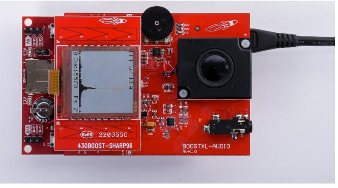
Figure 6. Stacked LaunchPad and BoosterPacks Reference Design
