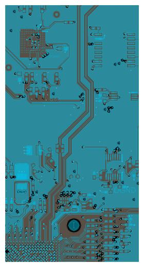
Figure 7. K2G GP EVM PCIe Reference Plane
