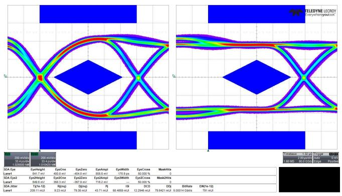
Figure 3 shows the K2G General Purpose EVM PCIe signal quality.
