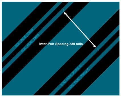
Figure 6. K2G GP EVM Inter-Pair Spacing
