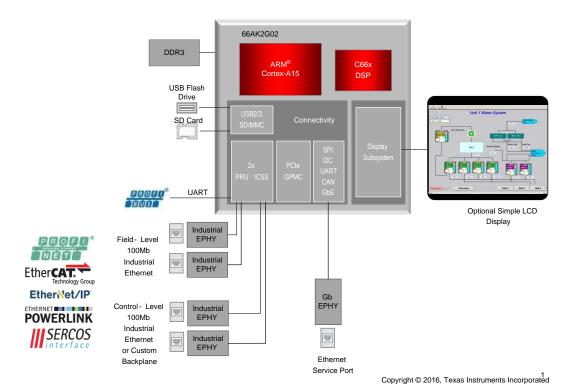
Figure 1. Industrial PLC System Block Diagram
