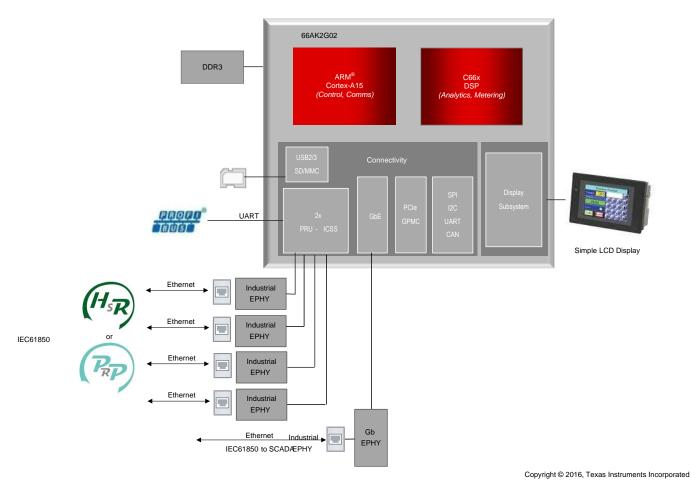
Figure 2. Protection Relay System Block Diagram
