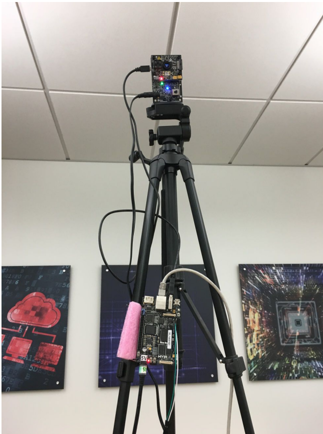
Figure 26. OPT8241 CDK and Rico Board on Tripod
