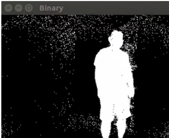
Figure 10. Background Subtraction Binary Image
