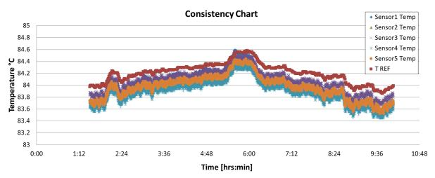
Figure 23. Temperature Consistency Test Result Under 85°C
