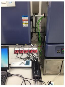
Figure 10. Test Setup With Humidity and Temperature Chamber
