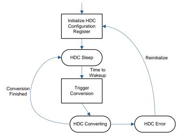
Figure 5. Flow Chart of HDC1080 Control
