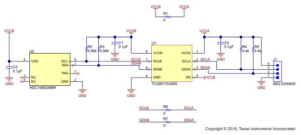
Figure 4. HDC1080 Sensor Board Schematic
