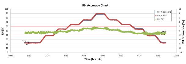
Figure 20. Humidity Accuracy Test Result Under 85°C
