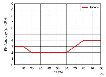
Figure 16. HDC1080 Humidity Accuracy Specification Versus Relative Humidity
