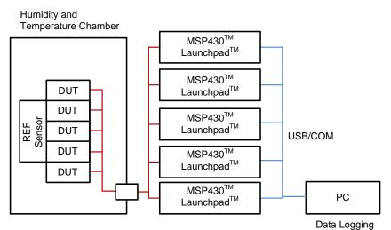
Figure 9. Test Setup Block Diagram
