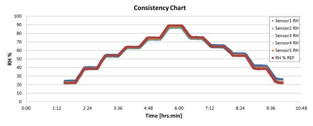
Figure 22. Humidity Consistency Test Result Under 85°C
