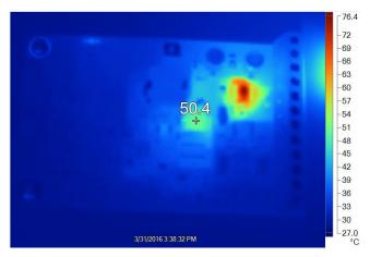
Figure 33. TPS40210-Q1 Boost-Converter Temperature Above 50°C at Three Strings of LEDs at 100 mA
