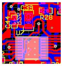
Figure 59. Input and Output Capacitor Placement
