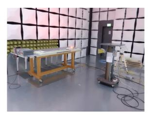
Figure 51. Radiated Emissions Setup With a Horn Antenna: 1.447 GHz to 1 GHz
