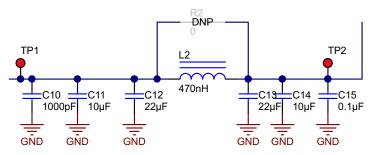
Figure 16. Input Voltage-Noise Filtering (R2 is Optional)
