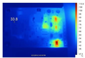
Figure 34. LM74610-Q1 Smart-Reverse Battery-Diode Temperature at 13.5-V Input Voltage
