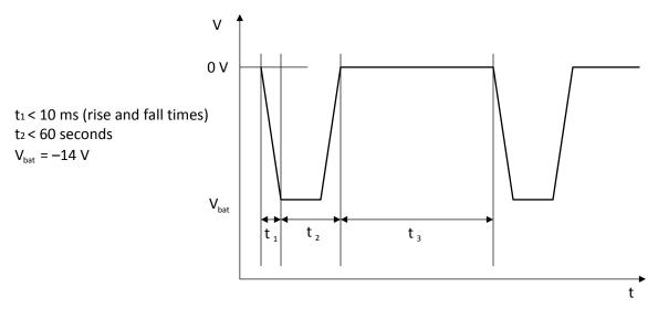
Figure 10. Reverse-Battery Pulse
