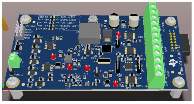
Figure 12. 3D Render of the TIDA-00678 Board
