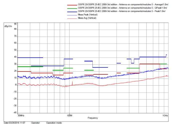
Figure 52. Ambient-Noise Level of Radiated Emissions: Line Side 30 MHz to 1 GHz
