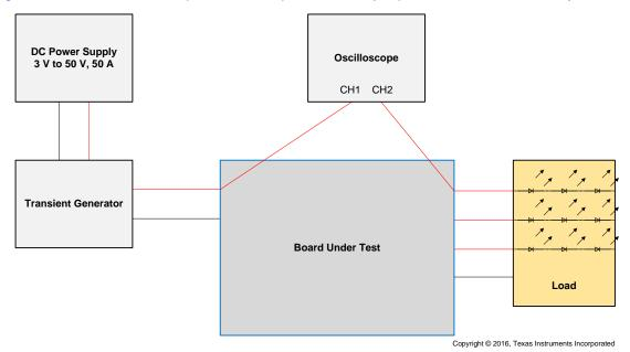
Figure 28. Test Setup for Load Dump, Cold Crank, Jump Start, and Reverse Battery
