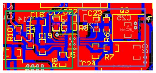
Figure 57. Switching-Converter Routing
