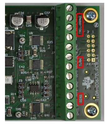
Figure 22. Screw Terminals for LED-String Outputs (100 mA and 150 mA, Maximum of 9 Strings, Maximum Output Voltage of 16.5 V)
