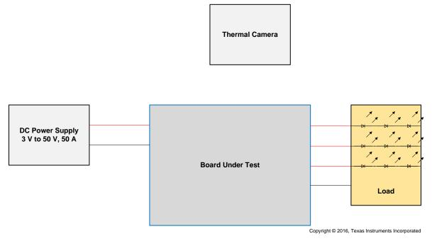
Figure 30. Setup to Measure Thermal Behavior of the Board
