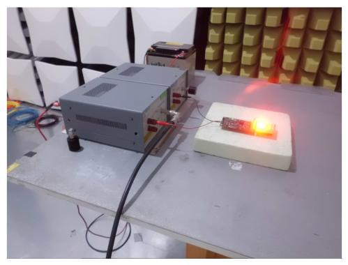
Figure 45. Conducted-Emissions Setup
