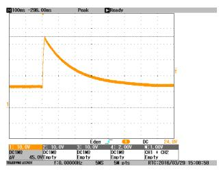
Figure 36. ISO 7637-2:2004 Pulse 4 Load Dump
