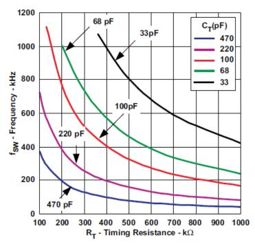
Figure 15. Switching Frequency versus Timing Resistance
