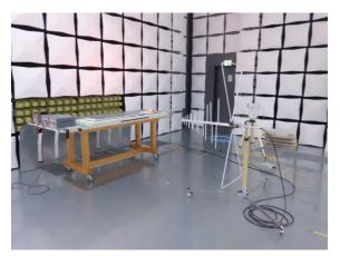
Figure 50. Radiated Emissions Setup With a Logarithmic Antenna: 30 MHz to 2.5 GHz
