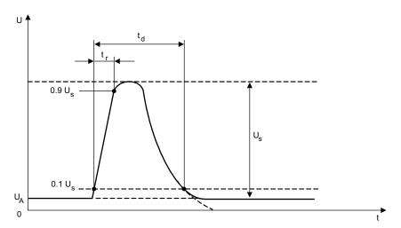
Figure 8. Load-Dump Pulse
