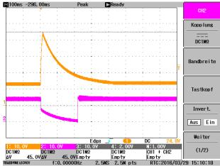
Figure 39. Load Dump and Output of TPS92630-Q1: Turned Off at > 17 V then Turned On
