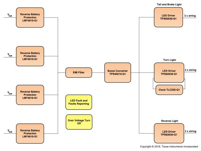
Figure 2. Step-Up and Linear LED Driver Block Diagram
