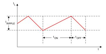
Figure 17. Input-Current Waveform
