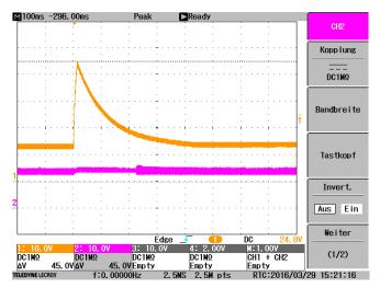
Figure 37. Load Dump (Orange) and Output (Pink) of TPS92630-Q1: No Turnoff
