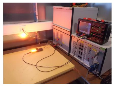
Figure 29. Setup for Transient Tests With LED Board and NSG 5500 Transient Generator
