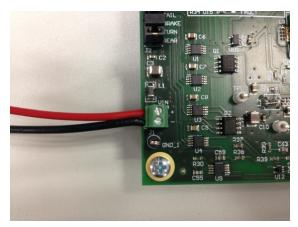
Figure 25. Board Supply-Input Terminal
