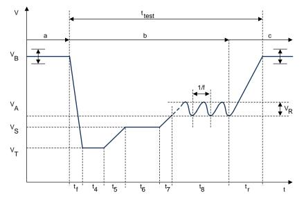
Figure 43. Cold-Crank Wave Shape
