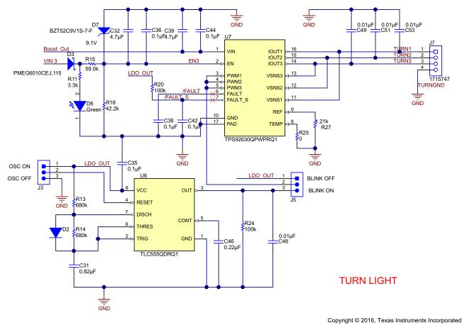
Figure 20. TPS92630-Q1 3-Channel LED Driver
