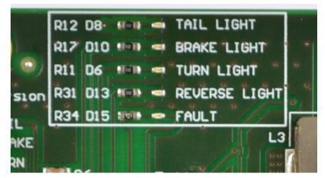
Figure 26. LEDs Indicating Failures and On Lights
