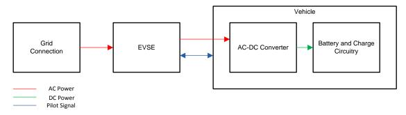
Figure 1. EVSE Position in Power Flow
