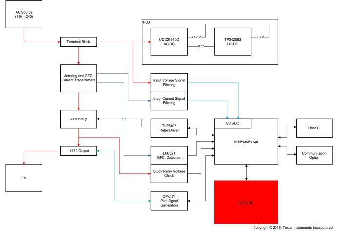
Figure 2. TIDC-EVSE-WiFi<sup>®</sup> Block Diagram
