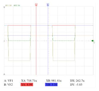
Figure 10. Pilot Signal TINA-TI™ Software Simulation
