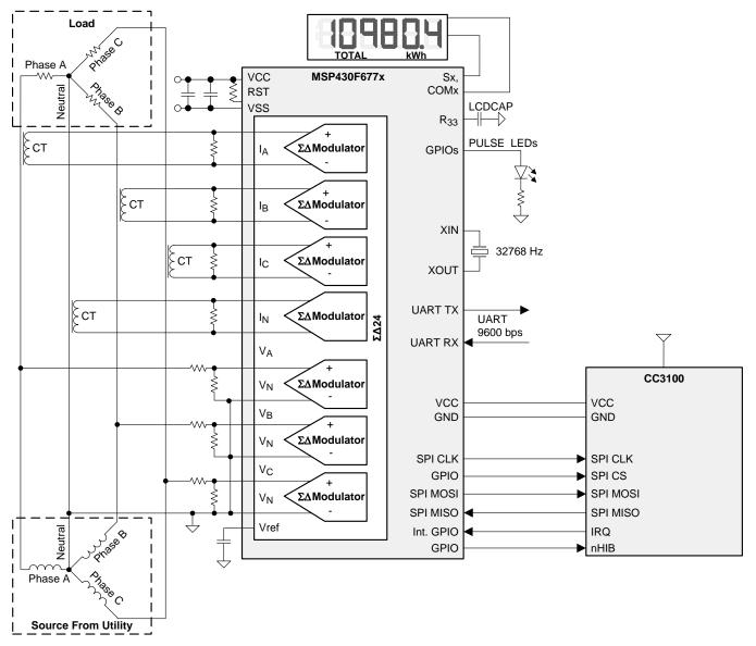
Figure 29. TIDC-3PHMTR-WIFIXR System Block Diagram
