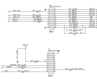
Figure 20. Connections on CC3100\_EM\_BP\_ADAPTER EM Female Connectors
