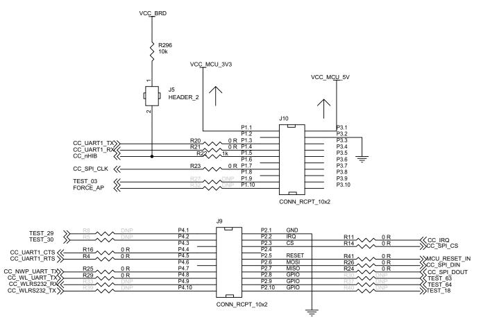
Figure 22. Connections on CC3100BOOST BoosterPack Female Connectors
