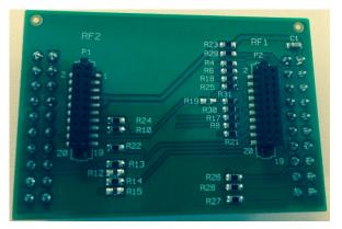
Figure 17. CC3100\_EM\_BP\_ADAPTER EM Female Connection
