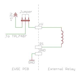
Figure 15. Normal Relay Connection
