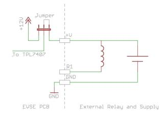
Figure 16. Relay With External Supply
