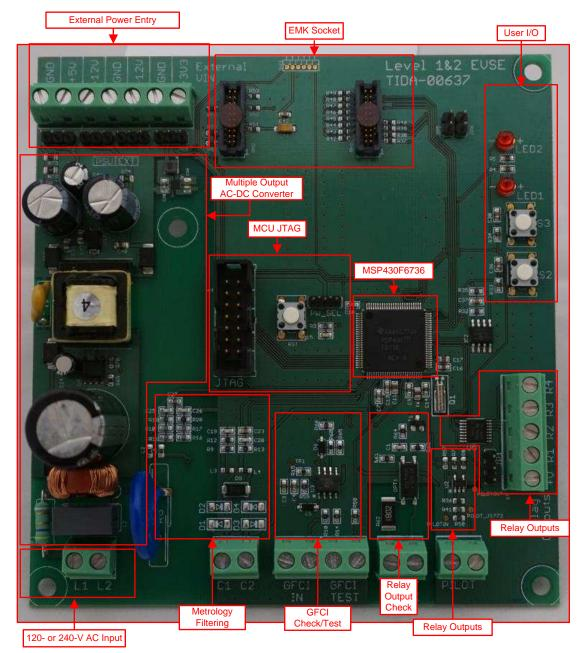
Figure 12. Top View of EVSE PCB
