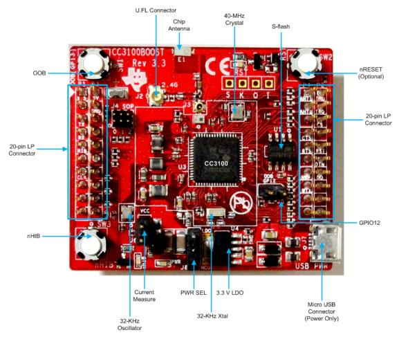
Figure 14. Front View of CC3100BOOST With Highlighted Components
