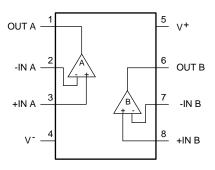
Figure 7. LM7322 Package Layout
