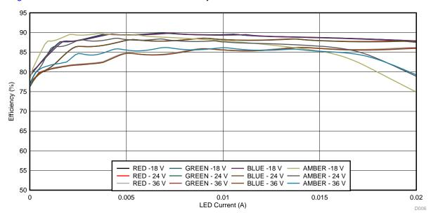
Figure 20 shows the DC-DC converter efficiency versus the LED current.
