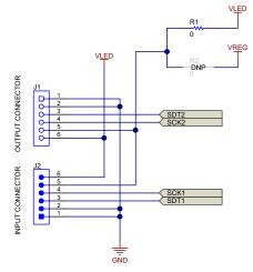
Figure 15. Connector and Power Options of LED Control Board
