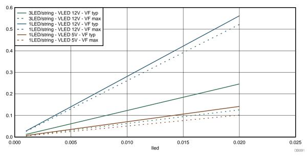
Figure 14. Power Dissipation in TLC5971 Versus LED current for Different Topolgies
