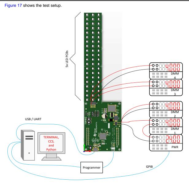
Figure 17. Test Setup
