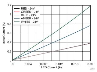
Figure 18. Input Current for Different LED Currents and LED Color
