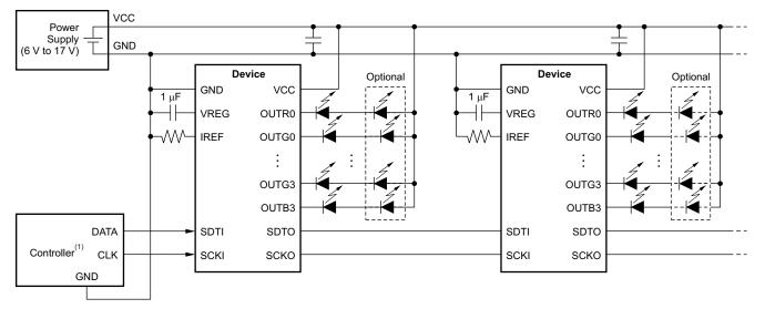
Figure 11. Example of Typical Application Circuit of TLC5971
