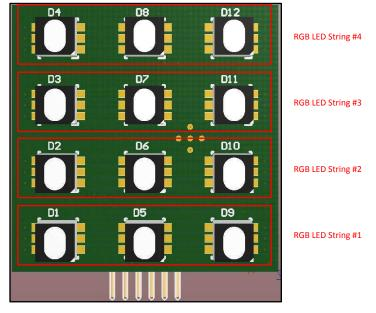
Figure 10. RGB LED Matrix PCB
