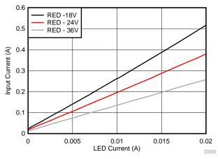
Figure 19. Input Current for Different LED Currents and Input Voltages
