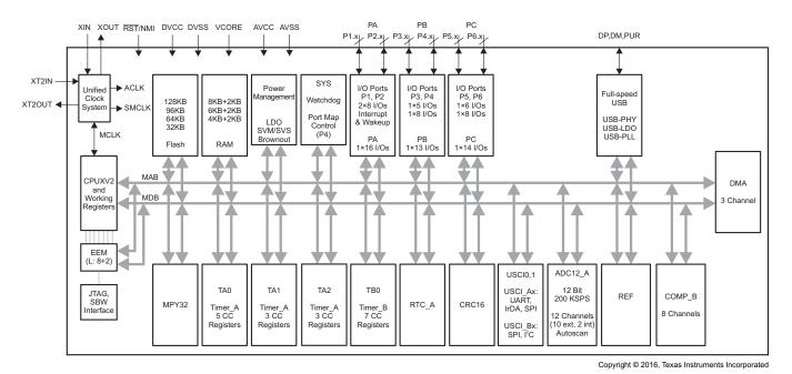
Figure 4. MSP430F5528 Functional Block Diagram
