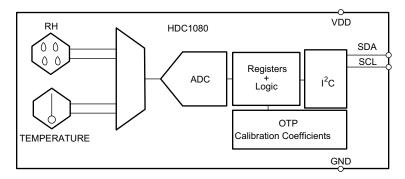
Figure 5. HDC1080 Functional Block Diagram
