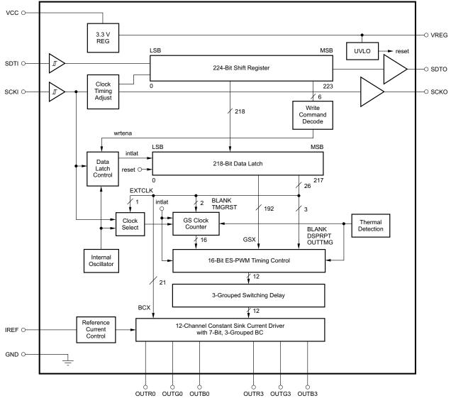
Figure 2. TLC5971 Functional Block Diagram
