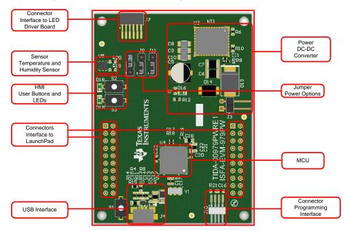
Figure 8. Power and Control Board
