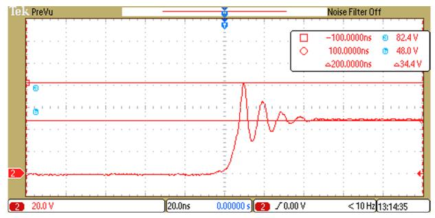
Figure 11. Voltage Waveform Across Drain Source of Low-Side MOSFET Without 25- $\Omega$  Gate Resistor, Peaking at 82.4 V
