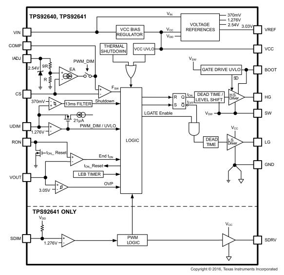
Figure 3. TPS92640, TPS92641 Block Diagram
