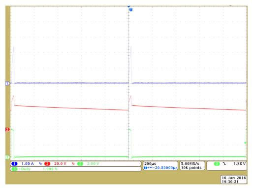
Figure 27. LED Current, LED Voltage, and UDIM Input Waveforms at 2% Duty Cycle
