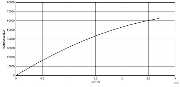
Figure 24. Illuminance versus I<sub>out</sub> (A)
