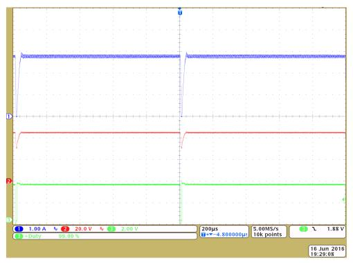
Figure 25. LED Current, LED Voltage, and UDIM Input Waveforms at 99% Duty Cycle
