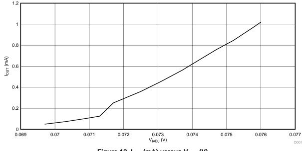
Figure 12. I<sub>OUT</sub> (mA) versus V<sub>IADJ</sub> (V)
