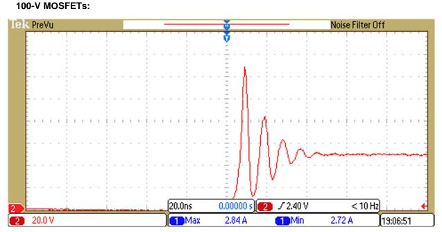
Figure 10. Voltage Waveform Across Drain Source of Low-Side MOSFET Without Any Gate Resistor, Peaking Around 124 V
