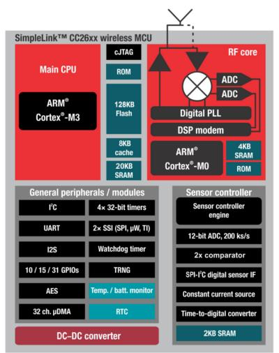
Figure 5. CC2650 Block Diagram
