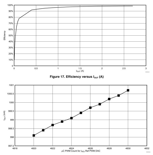
Figure 18. I<sub>OUT</sub> (A) versus µC Counts
