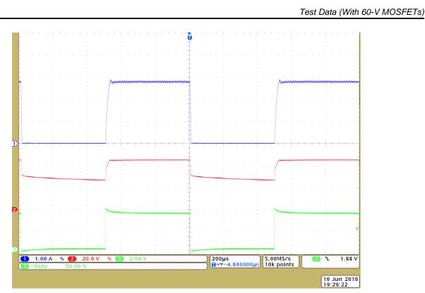
Figure 26. LED Current, LED Voltage, and UDIM Input Waveforms at 50% Duty Cycle
