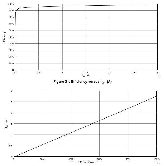
Figure 32. I<sub>OUT</sub> (A) versus UDIM Duty Cycle
