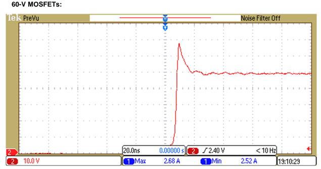
Figure 8. Voltage Waveform Across Drain Source of Low-Side MOSFET Without Any Gate Resistor, Peaking Around 68 V
