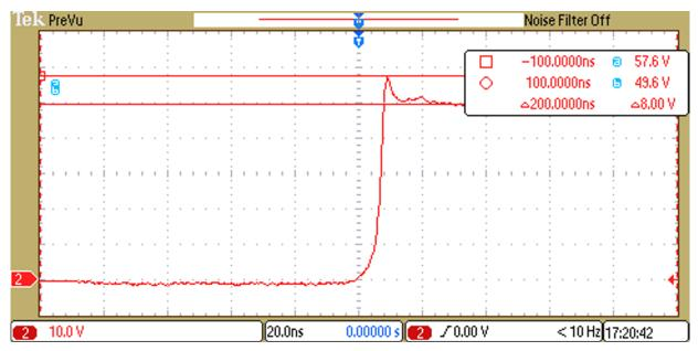
Figure 9. Voltage Waveform Across Drain Source of Low-Side MOSFET With 25- $\Omega$  Gate Resistor, Peaking at 57.6 V
