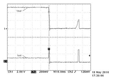
**Figure 18. Overcurrent Protection**
