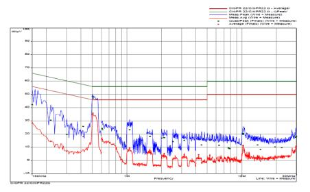
Figure 24. Conducted Emission Test Result with Filter (Wire +)
