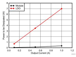
Figure 3. Comparison of Power Dissipated
