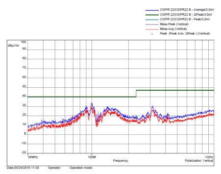
Figure 28. Radiated Emission 3-m Prescan Test Vertical Polarization
