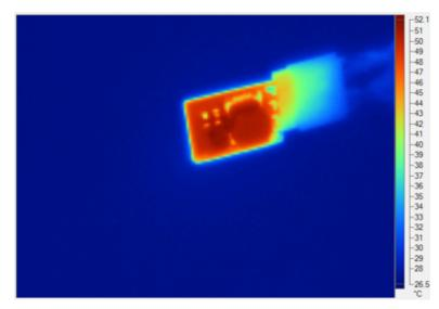
Figure 8. Bottom-Side Thermal Picture With 12-V $_{\rm IN},$  5 V at 1-A Output
