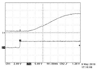
Figure 16. Start-up at 12-V Input and 1-A Output Load
