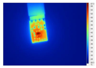
Figure 7. Top-Side Thermal Picture With 12-V<sub>IN</sub>, 5 V at 1-A Output
