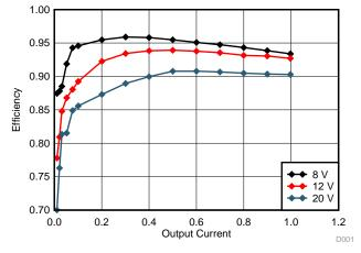
Figure 6. TIDA-00946 Efficiency
