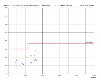
Figure 30. Radiated Emission 10-m Test Result
