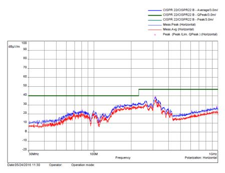
Figure 27. Radiated Emission 3-m Prescan Test Horizontal Polarization
