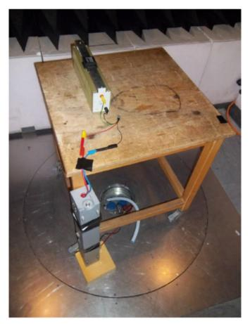
Figure 26. Radiated Emission 3-m Prescan Test Setup
