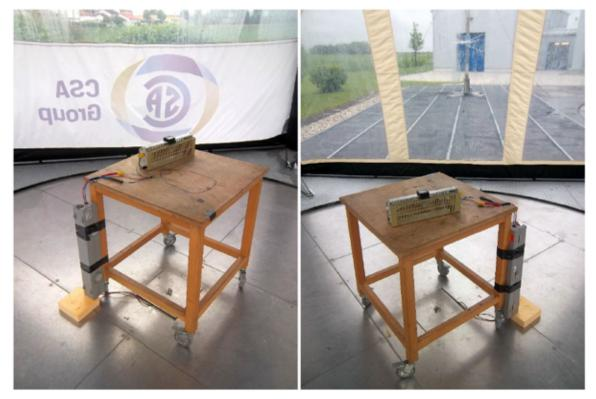
Figure 29. Radiated Emission 10-m Test Setup
