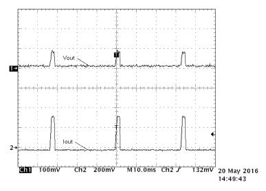
**Figure 19. Short-Circuit Protection**
