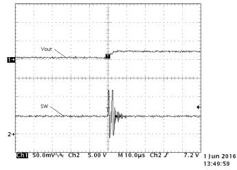
Figure 14. Output Voltage Ripple at No Load Output
