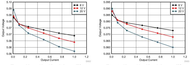
Figure 9. Line and Load Regulation at 65°C
