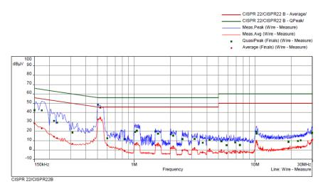
Figure 25. Conducted Emission Test Result with Filter (Wire -)
