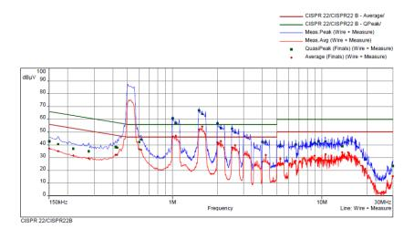
Figure 23. Conducted Emission Test Result Without Filter
