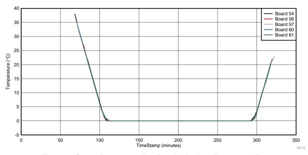
Figure 39. Sensor Temperature Readings During Low Temperature Test
