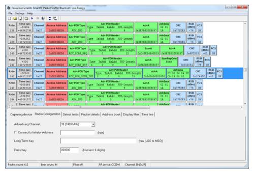
Figure 20. Packet Sniffer Software, Filterless Recording
