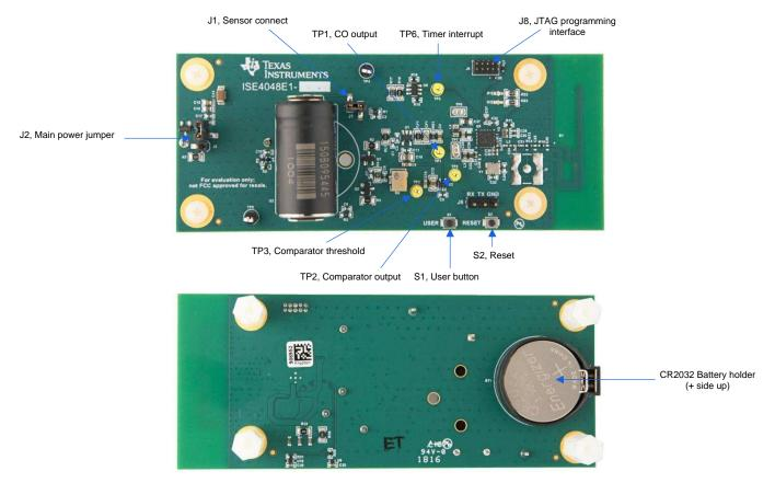
Figure 16. Low-Power Carbon Monoxide Sensor Reference Design Hardware Description
