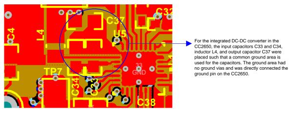
Figure 41. DC/DC Routing Guidelines
