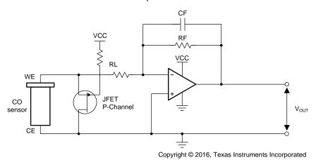
Figure 4. Sensor Anti-Polarization Technique Using P-Channel JFET
