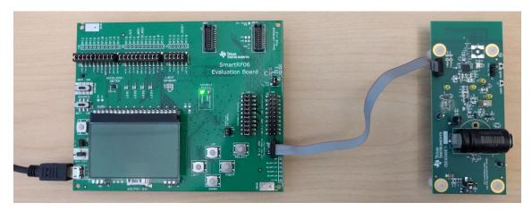
Figure 17. Connection of SmartRF06 EVM and TI Designs Hardware for Programming and Debugging
