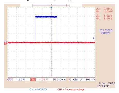
Figure 7. Sensor in Open Circuit
