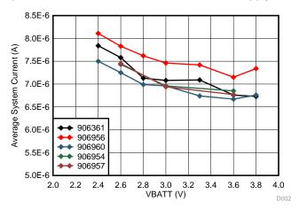
Figure 31. Pre-Alarm State Current Consumption Across System Voltage
