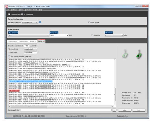
Figure 22. SmartRF Studio Packet Sniffer Recording
