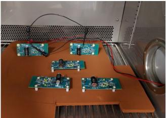
Figure 26. Temperature and Humidity Test Setup
