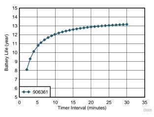
Figure 34. Battery Life versus Timer Interval
