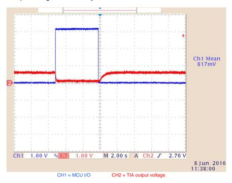
Figure 8. Sensor in Short-Circuit
