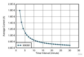
Figure 33. Combined Standby and Test State Average Current versus Timer Interval
