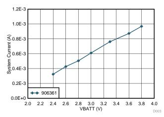
Figure 32. Alarm State Current Consumption Across System Voltage
