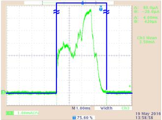
Figure 11. Power Profile During Startup Period
