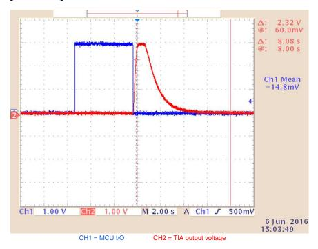
Figure 6. Normal Sensor Response to Test Current (With CO Gas)
