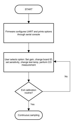
Figure 15. Calibration Procedure
