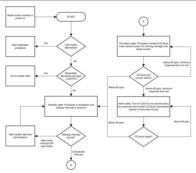
Figure 13. Normal Operation Flowchart
