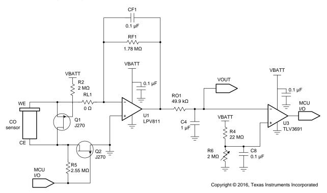
Figure 9. CO Sensor Analog Signal Path Schematic
