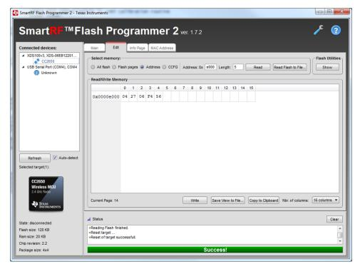
Figure 23. SmartRF Flash Programmer 2 Configuration for Loading Calibration Values
