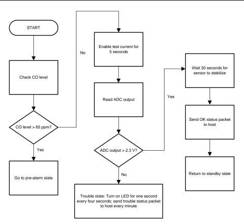
Figure 14. Sensor Test Procedure
