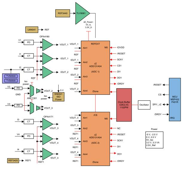
Figure 2. TIDA-00835 Block Diagram
