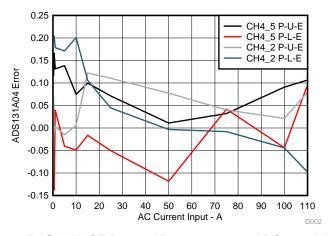
Figure 35. ISO\_V\_CT Power Measurement—ADC1 and ADC2
