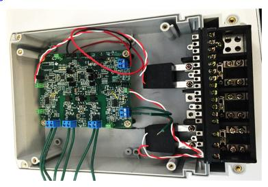
Figure 23. Data Acquisition AFE With External CTs
