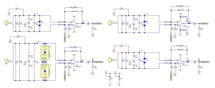
Figure 9. Current Input Connectors with Gain Amplifiers and Flat clamp TVS protection
