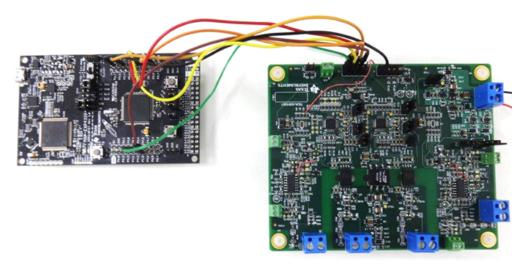
Figure 24. Data Acquisition AFE With MCU Interface
