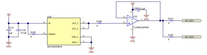
Figure 8. External Reference for ADC1 and ADC2
