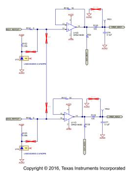
Figure 12. Reference With Buffer for Gain Amplifiers
