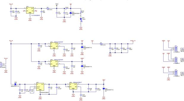
Figure 13. Onboard Positive and Negative Power Supply With Protection
