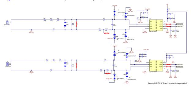
Figure 11. Isolation Amplifier With Input Protection and Potential Divider
